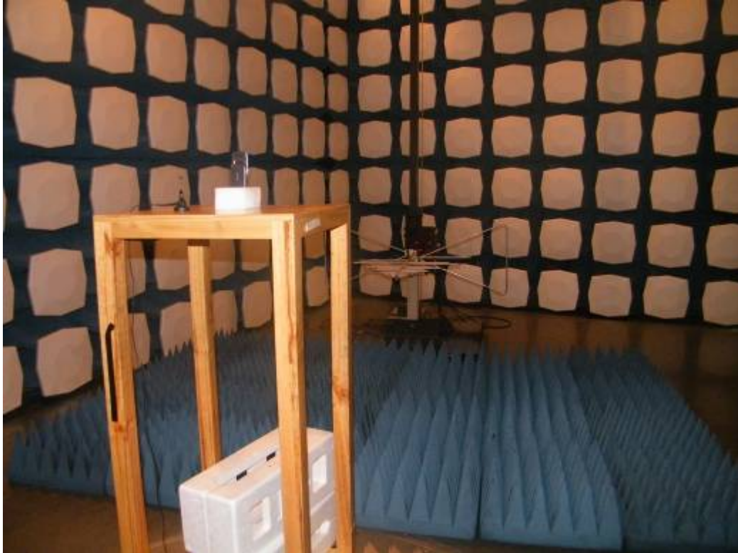
Picture 2: Radiated Spurious Emissions Test setup
