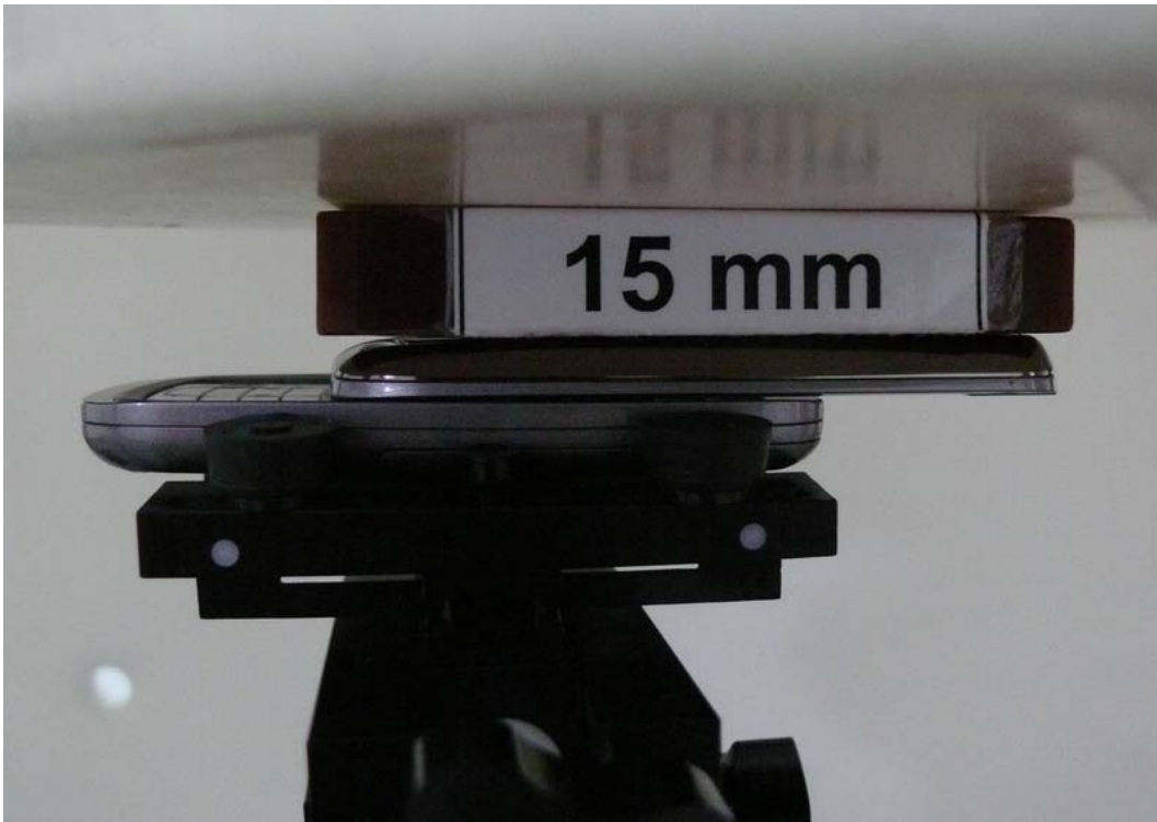
Picture 18: Body, The EUT display towards phantom, the distance from handset to the bottom of the Phantom is 15mm (The spacer was removed during testing, Slide Open)
