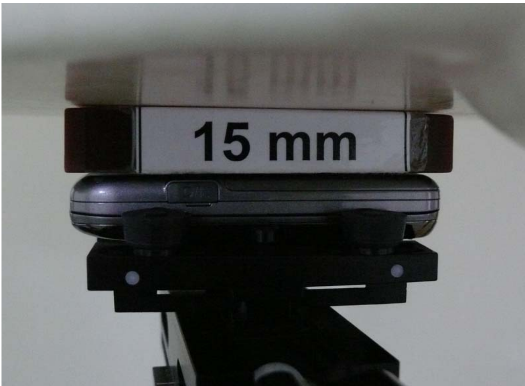
Picture 17: Body, The EUT display towards ground, the distance from handset to the bottom of the Phantom is 15mm (The spacer was removed during testing, Slide Close)
