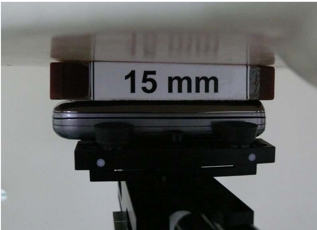
Picture 19: Body, The EUT display towards phantom, the distance from handset to the bottom of the Phantom is 15mm (The spacer was removed during testing, Slide Close)
