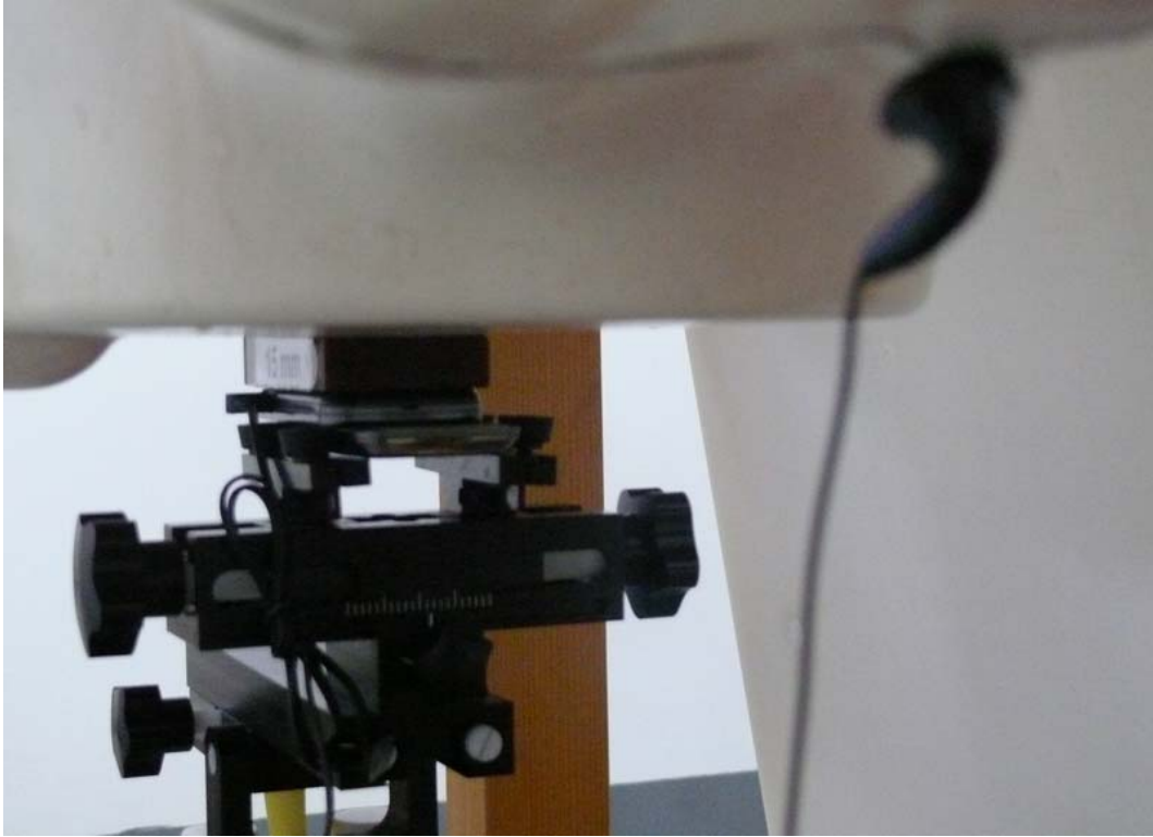
Picture 20: Body with earphone, The EUT display towards ground, the distance from handset to the bottom of the Phantom is 15mm (Slide Open)
