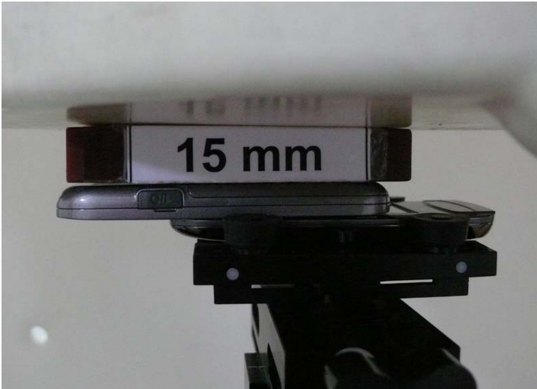
Picture 16: Body, The EUT display towards ground, the distance from handset to the bottom of the Phantom is 15mm (The spacer was removed during testing, Slide Open)
