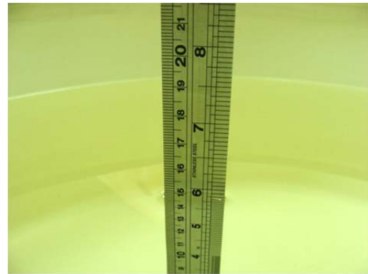
Fig 6.2 Photo of Liquid Height for Body SAR
