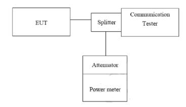
Measurement Setup for testing on Antenna connector.
