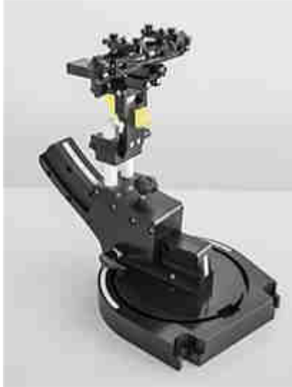
Mounting Device for Hand-Held Transmitters
