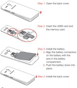
Always turn off your smartphone first before you insert or remove a USIM card. Insert or remove a USIM card with your smartphone on may damage your USIM card or smartphone permanently.
