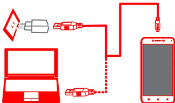
Connect your smartphone to a power outlet using the cable and USB power adapter that come with your smartphone.
