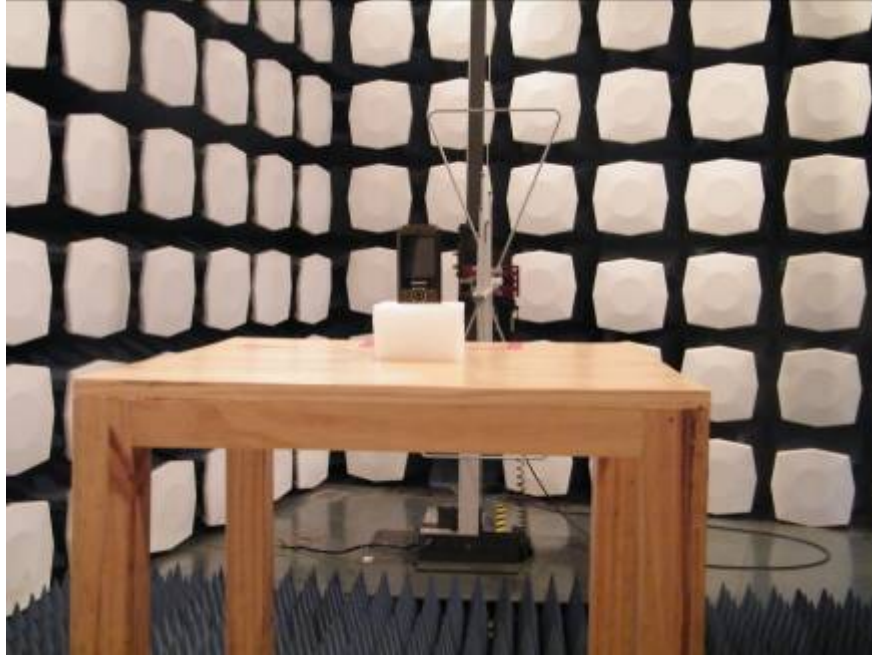
Picture 2: Radiated Spurious Emissions Test setup
