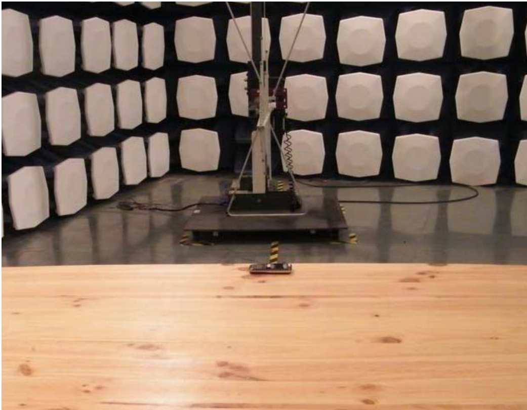
Picture 2 Radiated Emission Test Setup
