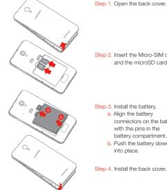
Step 2. Insert the Micro-SIM card and the microSD card.
