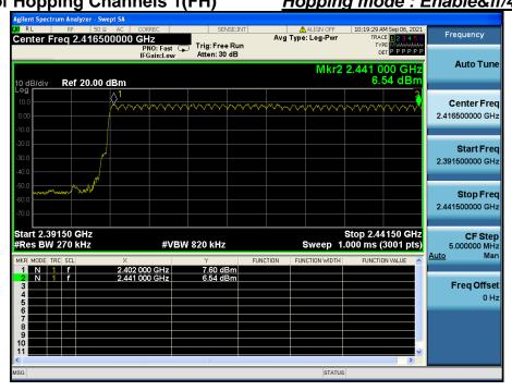
Number of Hopping Channels 2(FH) <u>Hopping mode : Enable &π/4DQPSK</u>
