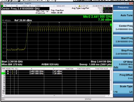
Number of Hopping Channels 2(FH) <u>Hopping mode : Enable & GFSK</u>
