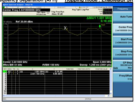
Carrier Frequency Separation (AFH) <u>Hopping mode : Enable&π/4DQPSK</u>
