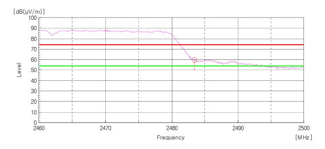
AV Detector: RBW: 1 MHz, VBW: 10 Hz (2 483.5 MHz - 2 500 MHz), Worst case (High, Horizontal)
