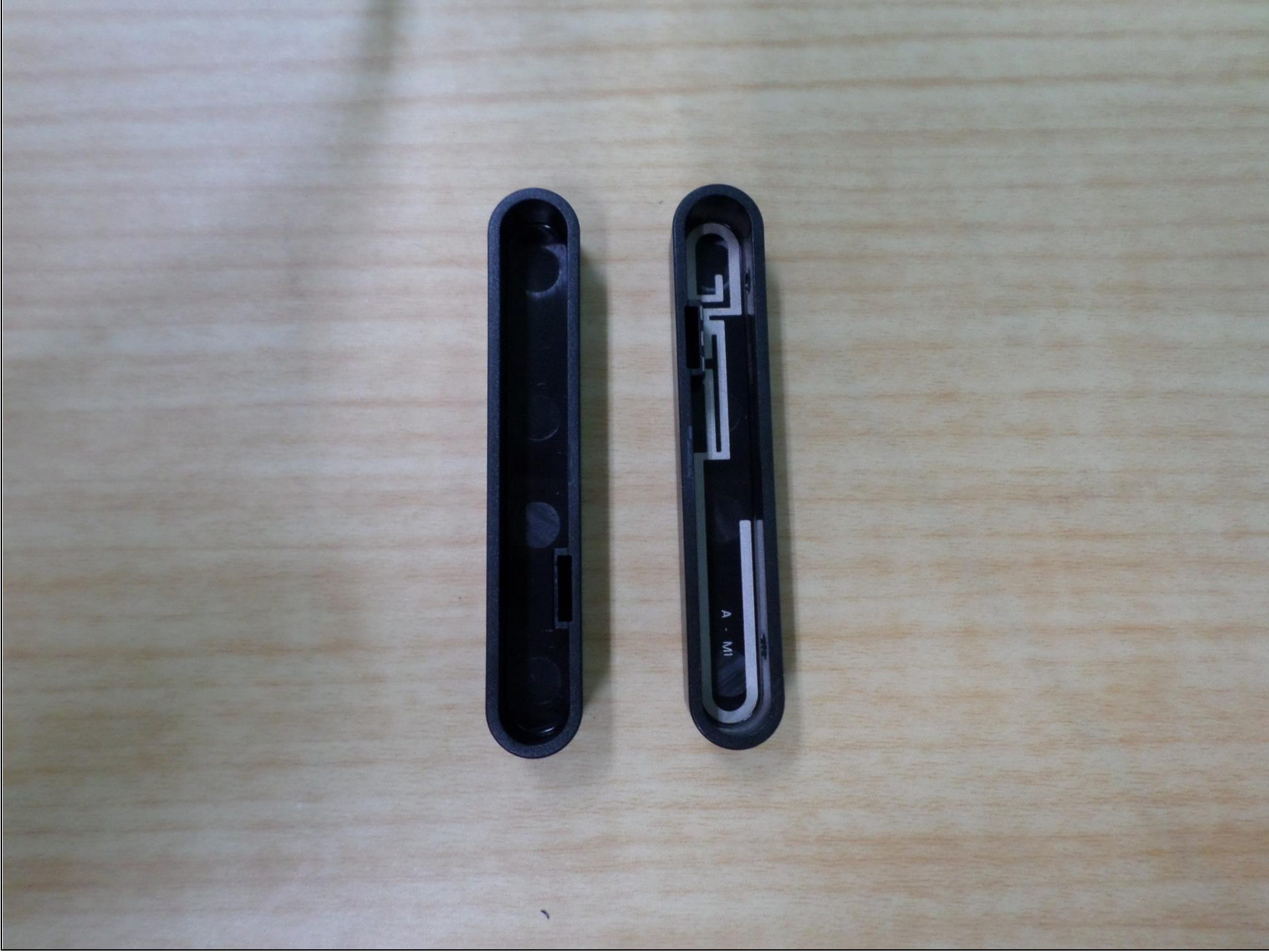
View of Antenna
