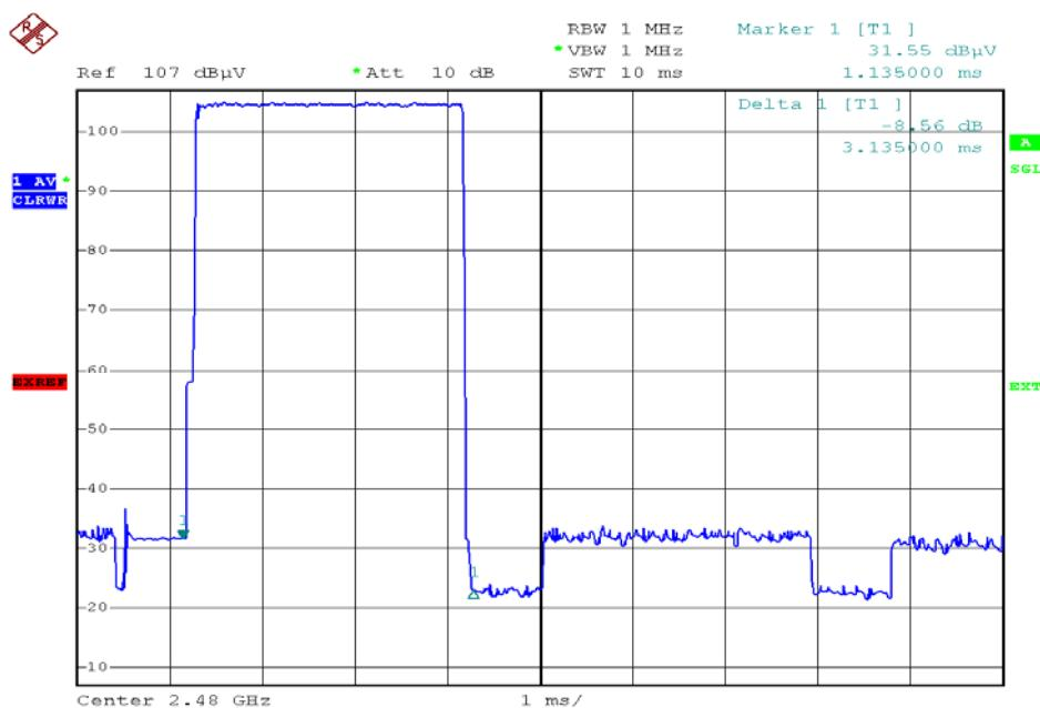
**Channel 78 2480 MHz DH3**
