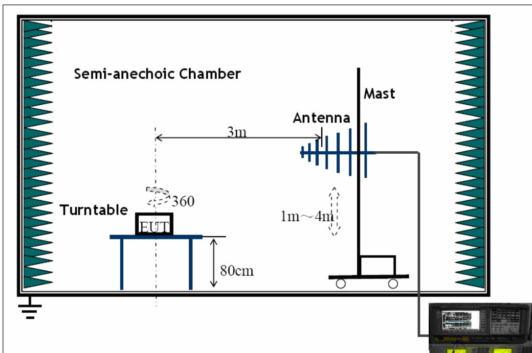
The EUT was placed on the test table in shielding room.
