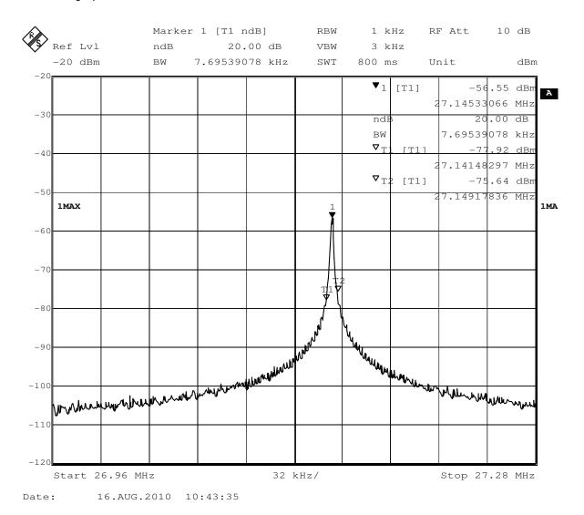
20dB bandwidth lower frequency: 27.14149297MHz 20dB bandwidth upper frequency: 27.14917836MHz
