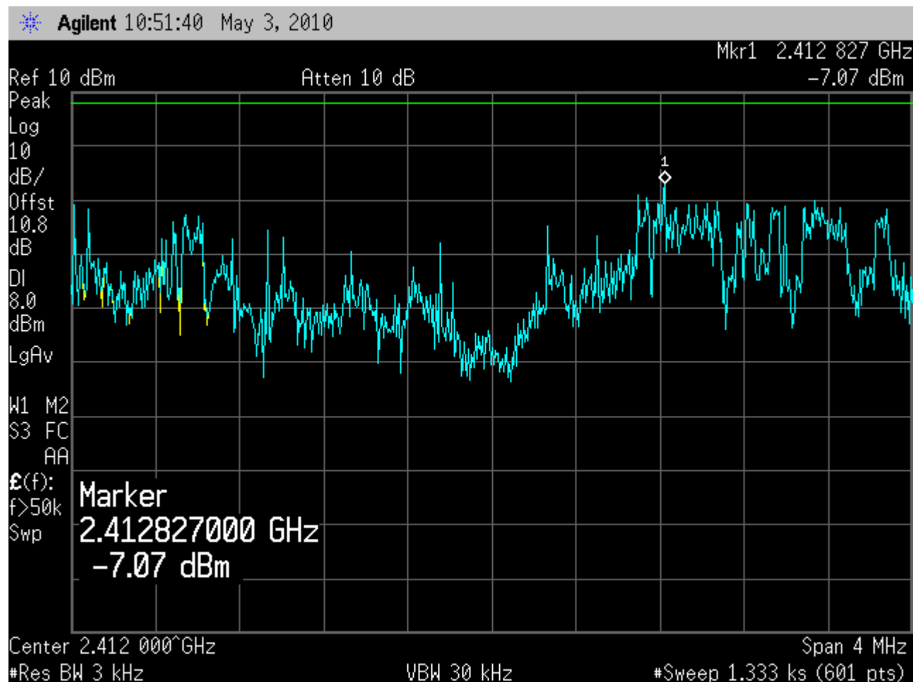
Low Channel ("g" mode) – Peak level is -7.07 dBm
