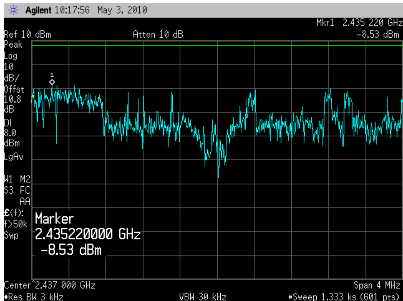
Mid Channel ("g" mode) – Peak level is -8.53 dBm
