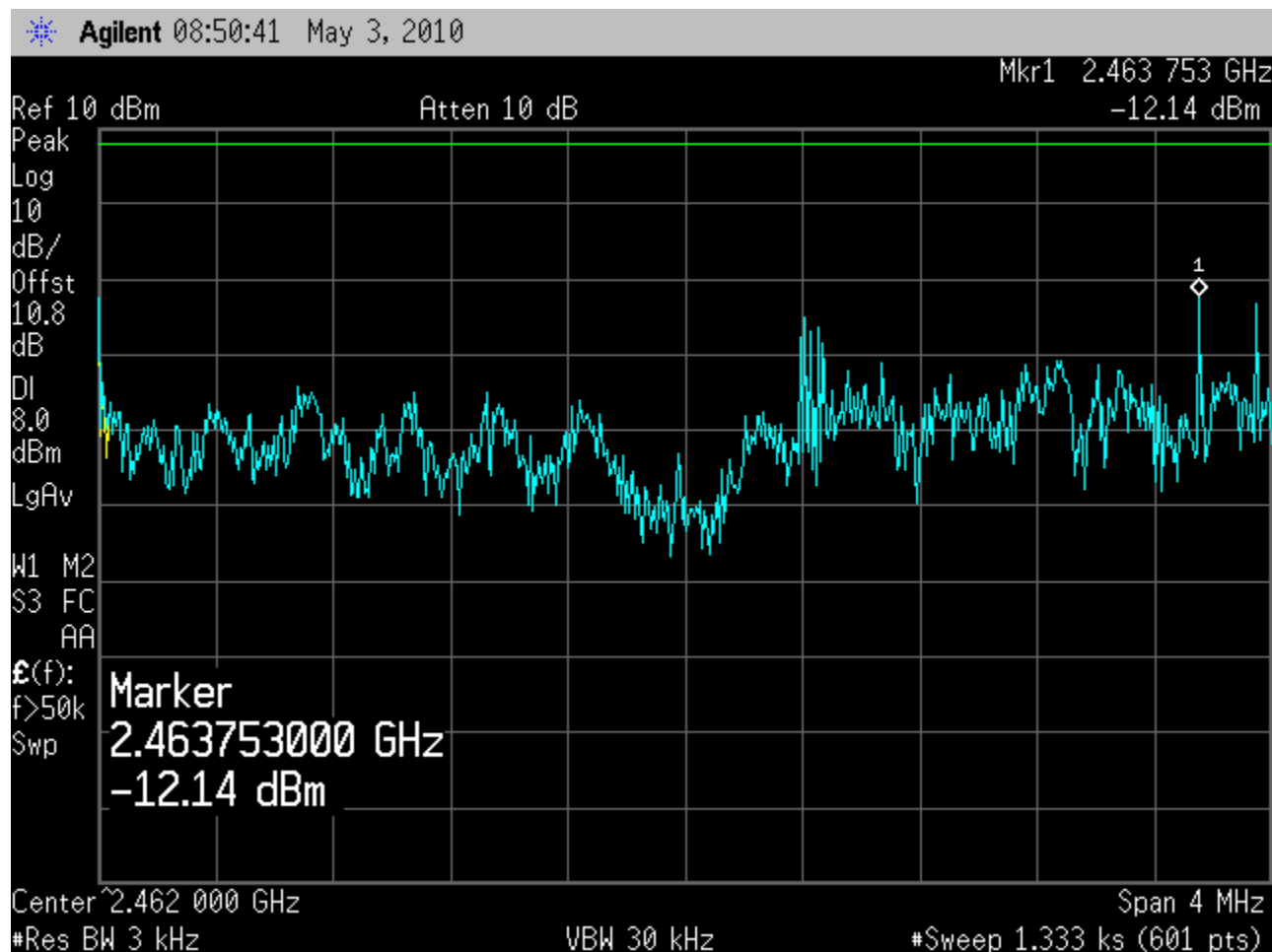
High Channel ("g" mode) – Peak level is -12.14 dBm
