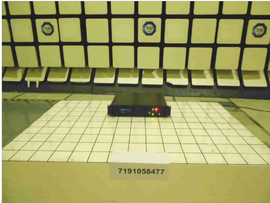
Radiated Emissions Test Setup (Front View)
