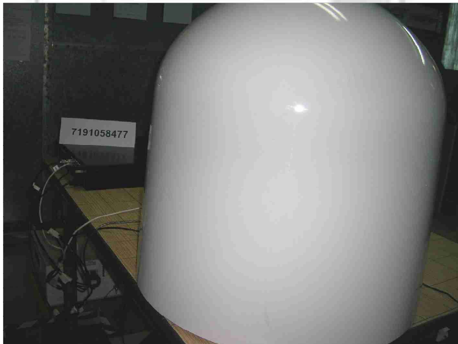
Conducted Emissions Test Setup (Rear View)
