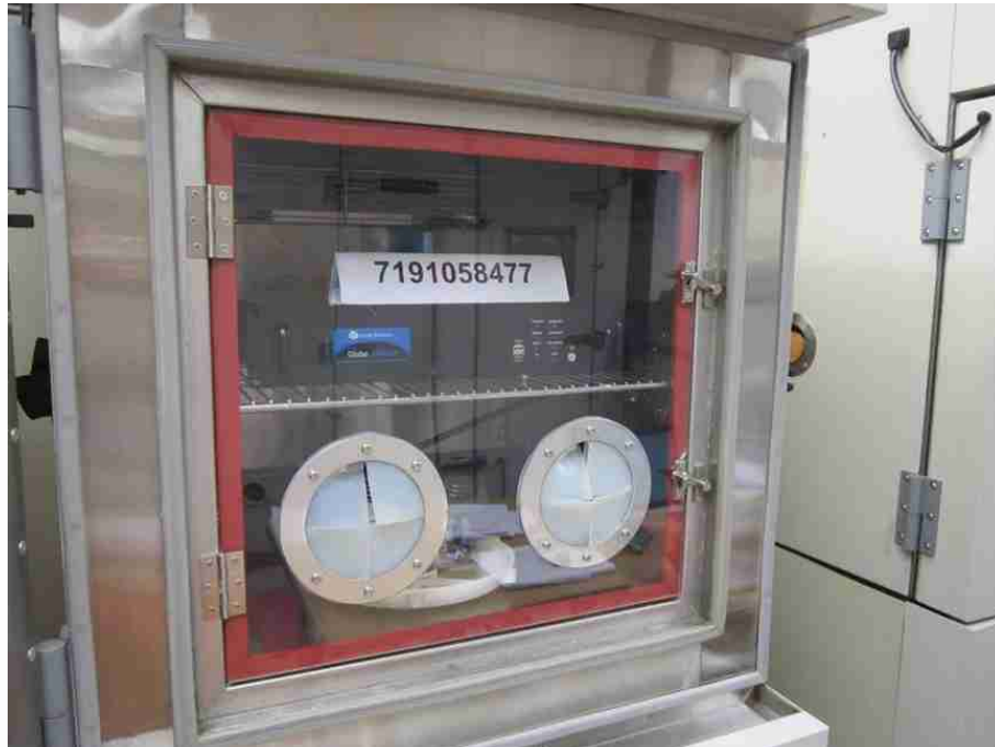
Frequency Stability (Temperature Variation) Test Setup
