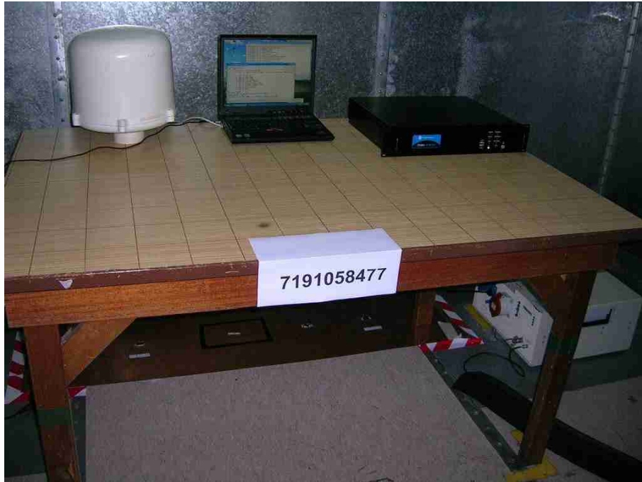
Conducted Emissions Test Setup (Front View)
