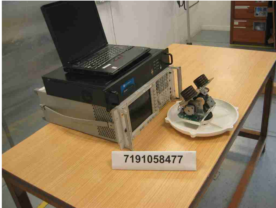
Unwanted Emissions at Antenna Terminal Test Setup
