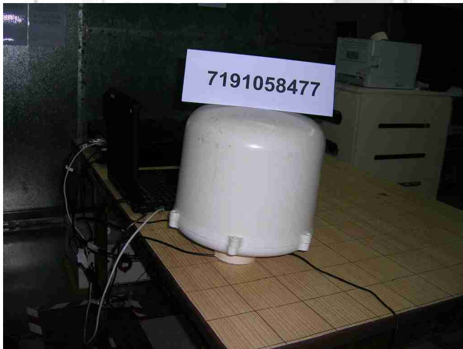
Conducted Emissions Test Setup (Rear View)
