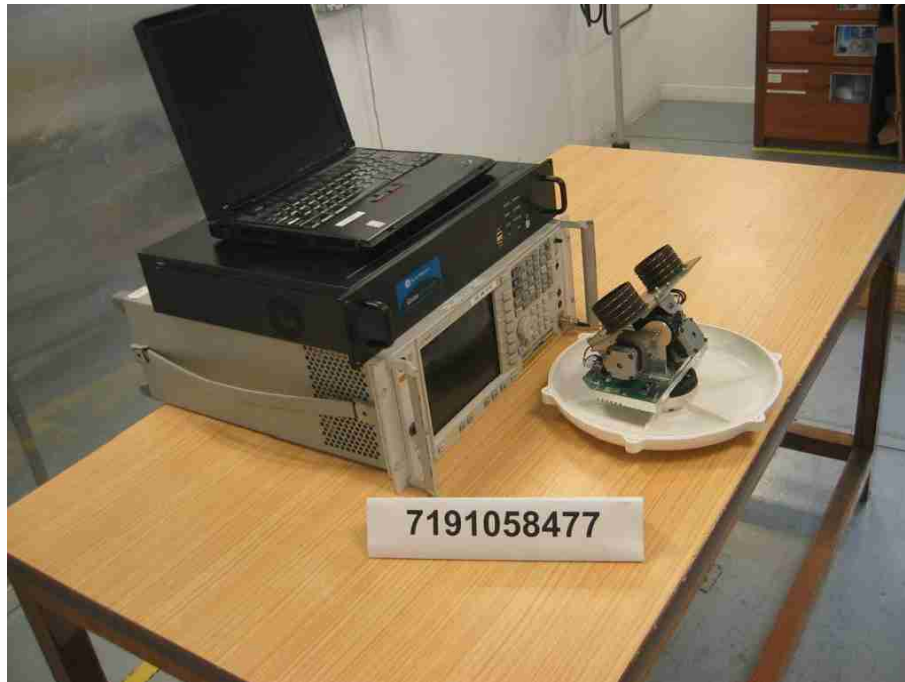
RF Output Power Test Setup
