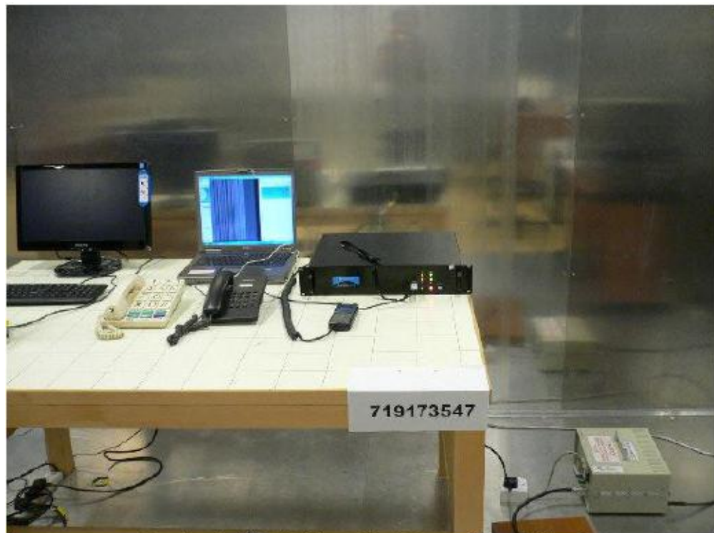
Conducted Emissions Test Setup (Front View)
