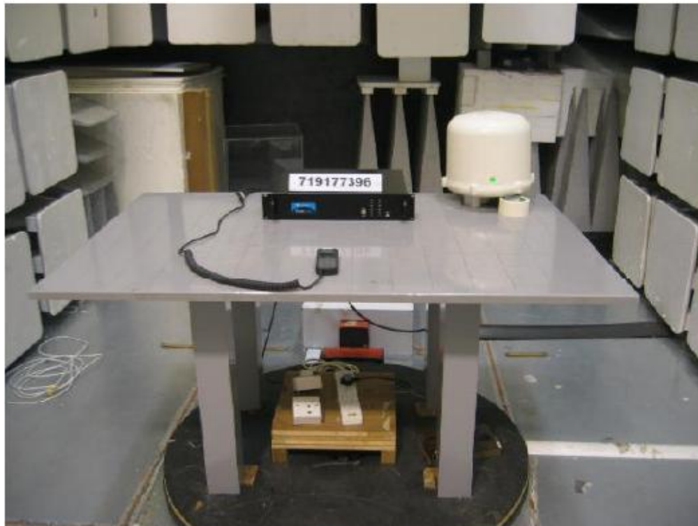
Radiated Spurious Emissions Test Setup (Front View)
