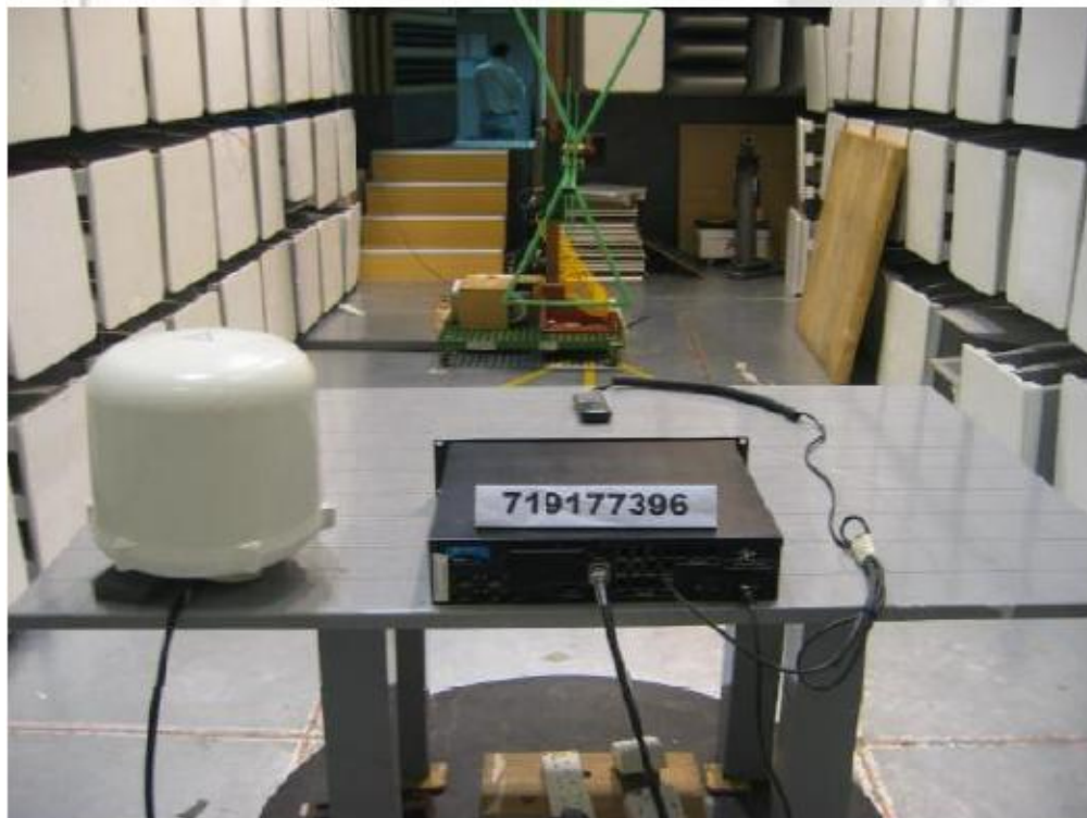
Radiated Spurious Emissions Test Setup (Rear View)
