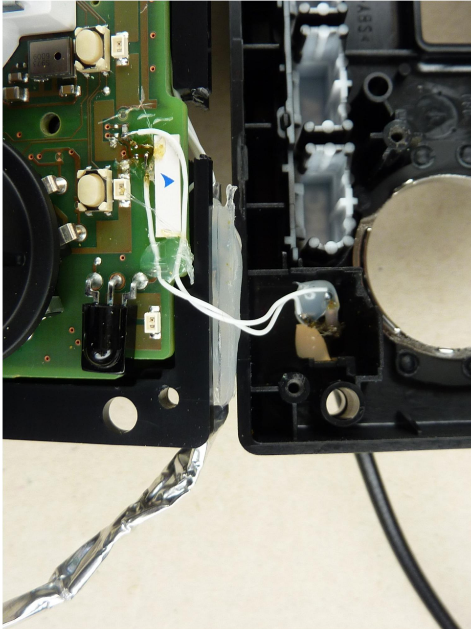
132962_19.JPG: Switch PCB, detail view to temporary antenna connector
