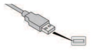
Insert the USB memory stick in the USB port or connect the USB device to the USB port using a suitable cable (not supplied).
