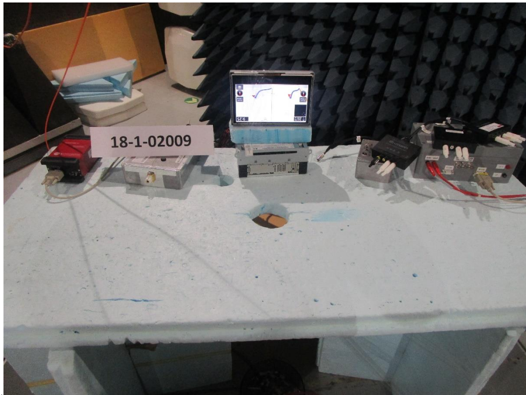
Photograph 1: Setup for Radiated emissions 30MHz-1GHz measurements, close view
