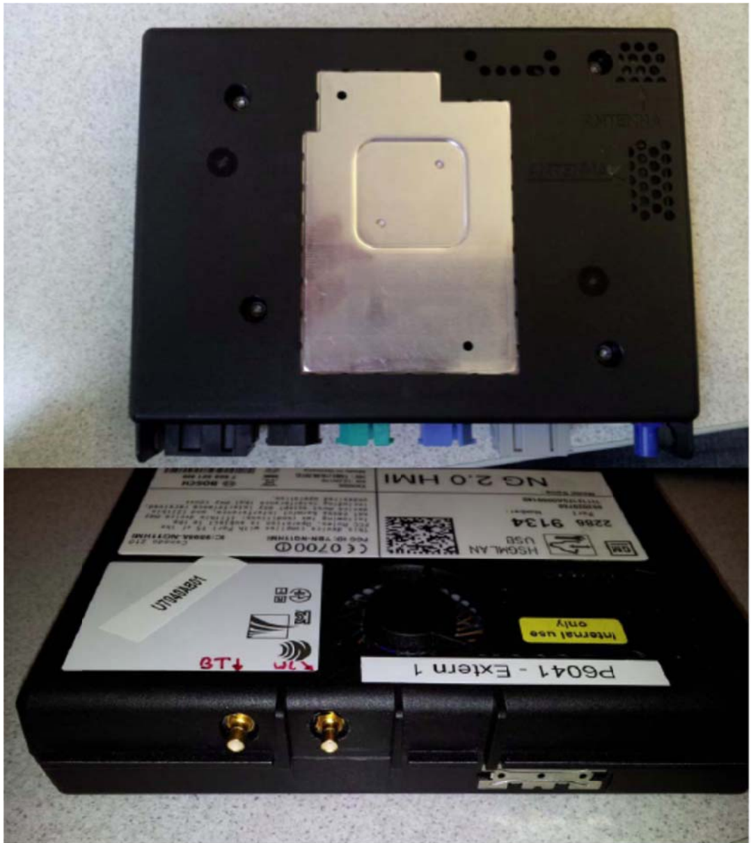
Photo with temporary antenna connectors for Bluetooth and WLAN.
