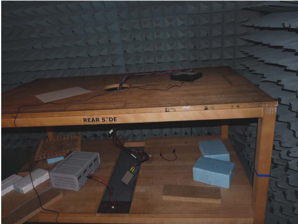
Photo 1: Test setup for radiated measurements (below 30 MHz)
