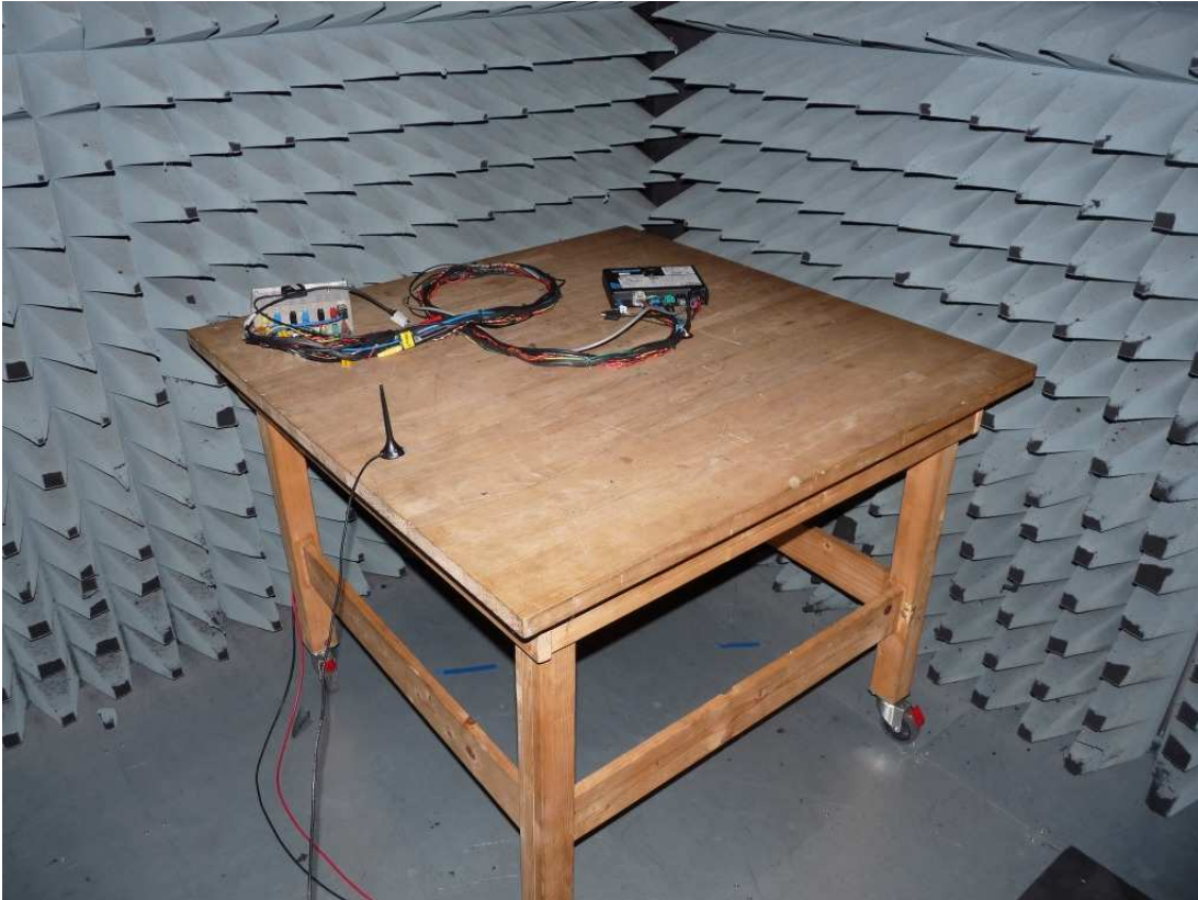
Photo 1: Test setup for radiated measurements (below 30 MHz)
