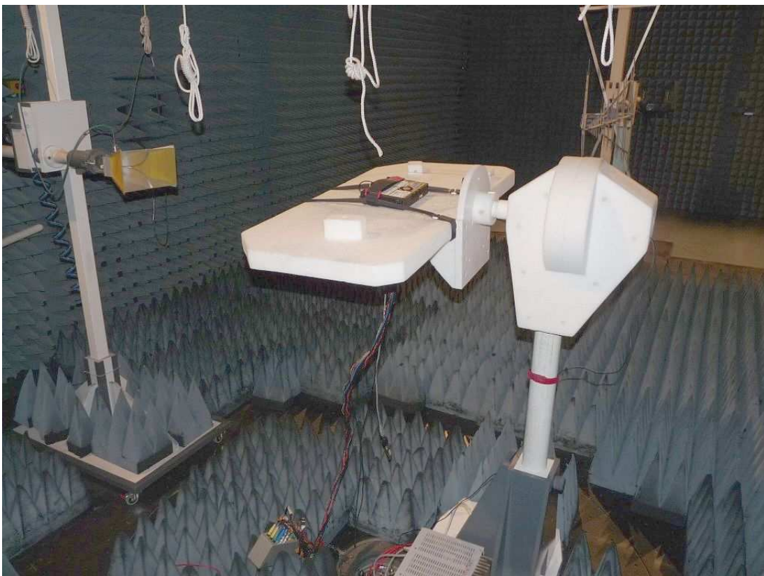
Photo 3: Test setup for radiated measurements (above 1 GHz)
