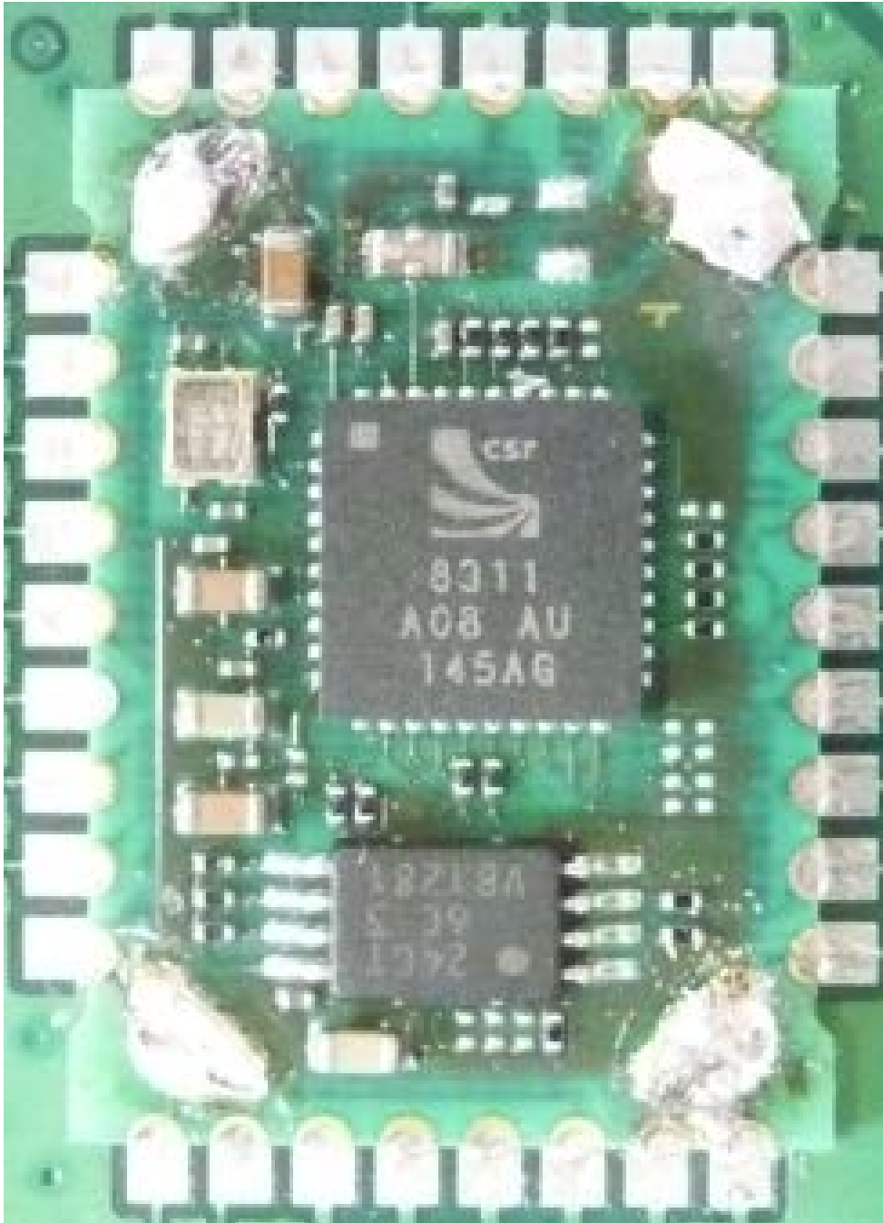
1.6. Photograph: Bluetooth Module on switchboard with removed shielding
