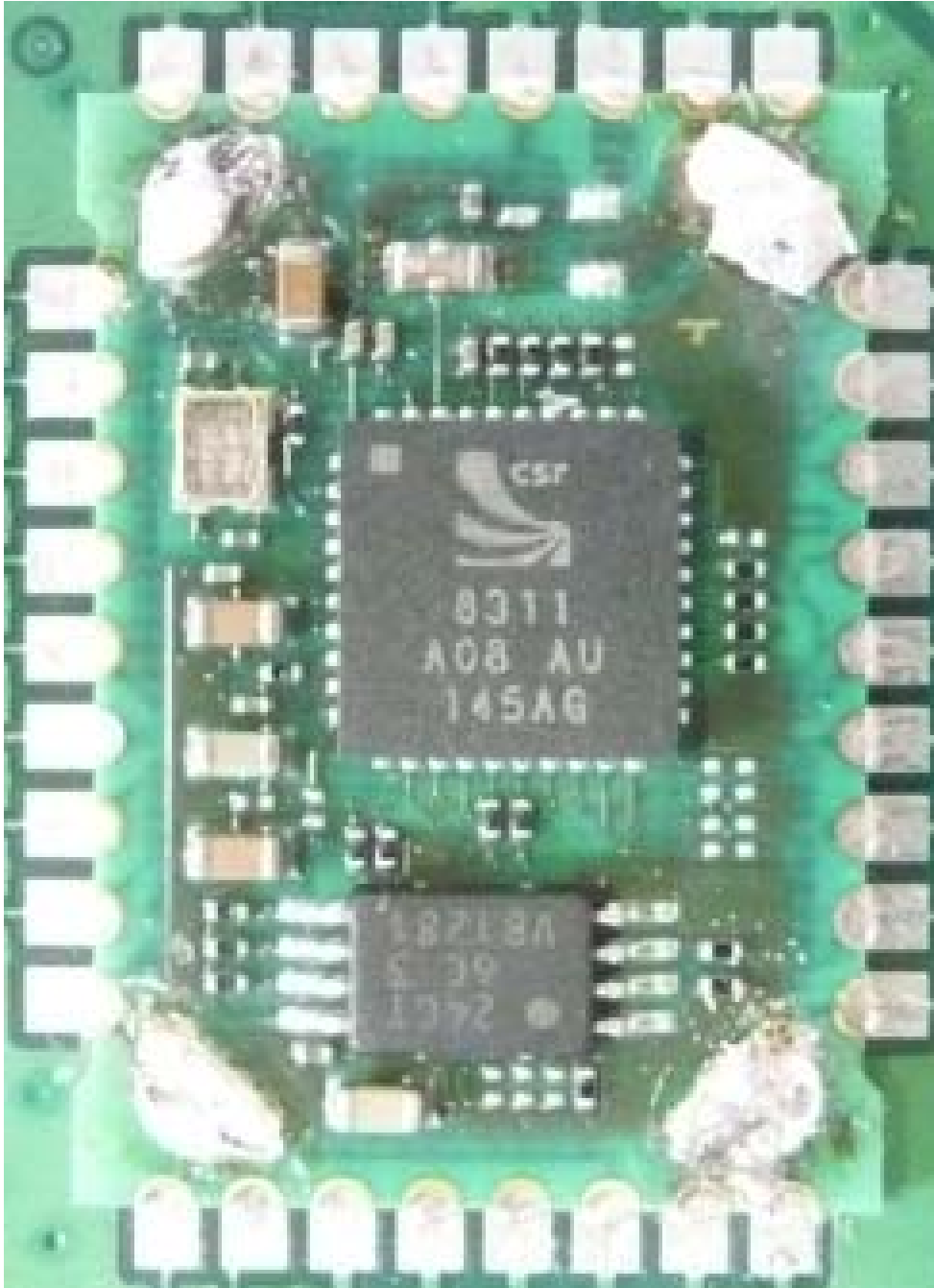
1.6. Photograph: Bluetooth module on switchboard with removed top shielding
