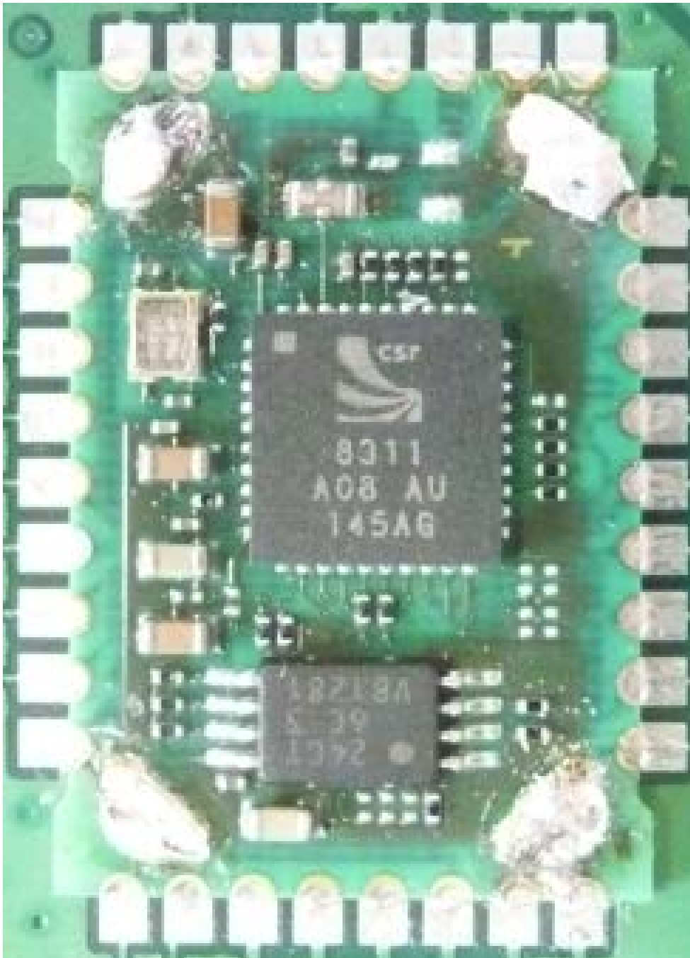
1.6. Photographs: BT Module on switch board with removed top shielding
