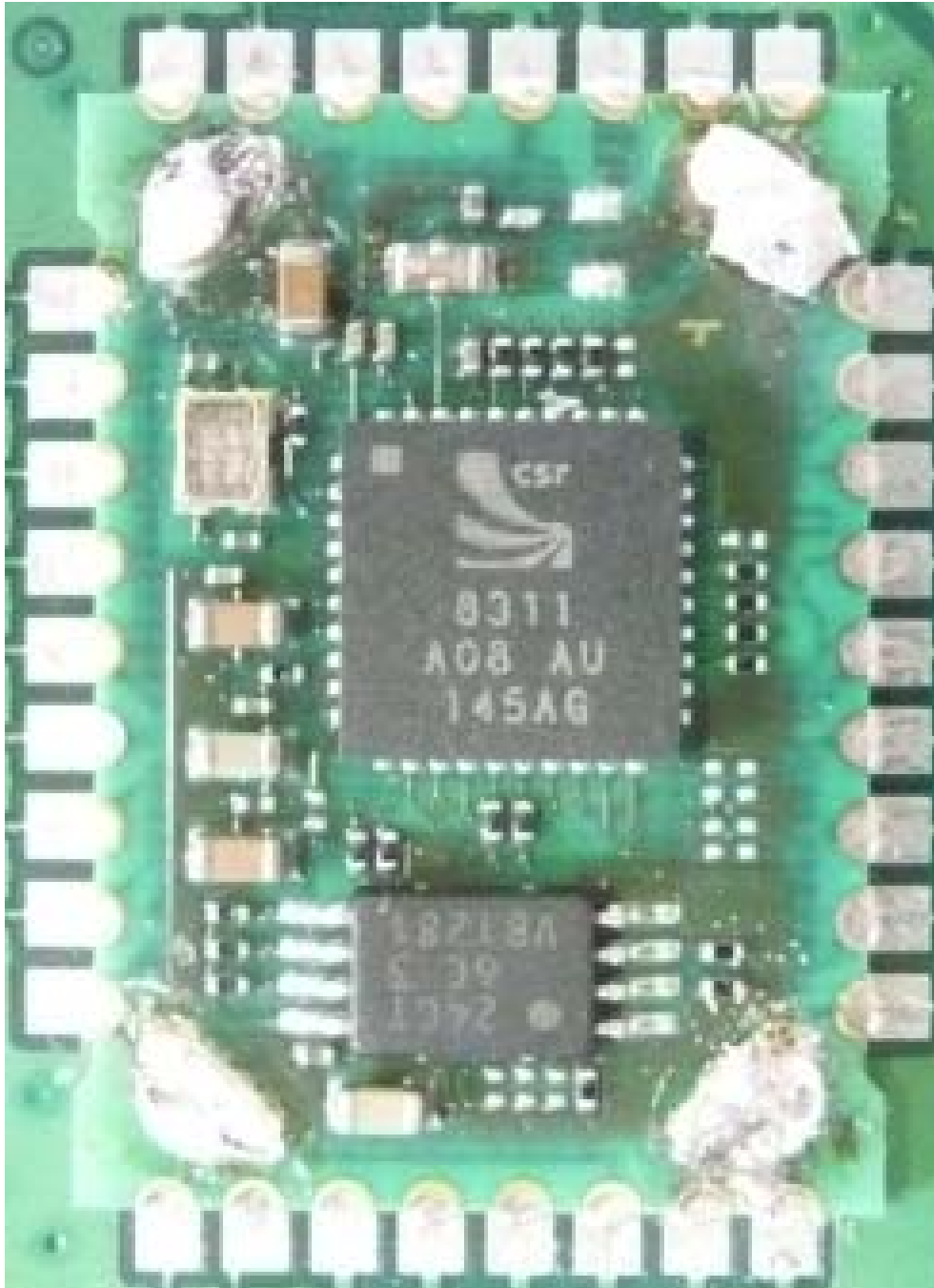
1.6. Photograph: BT-module on switchboard with removed top shielding
