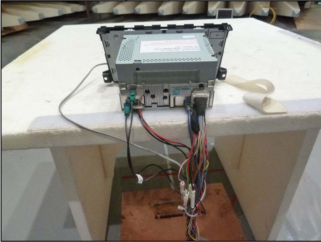
Photo 3: wiring of the setup of radiated emission
