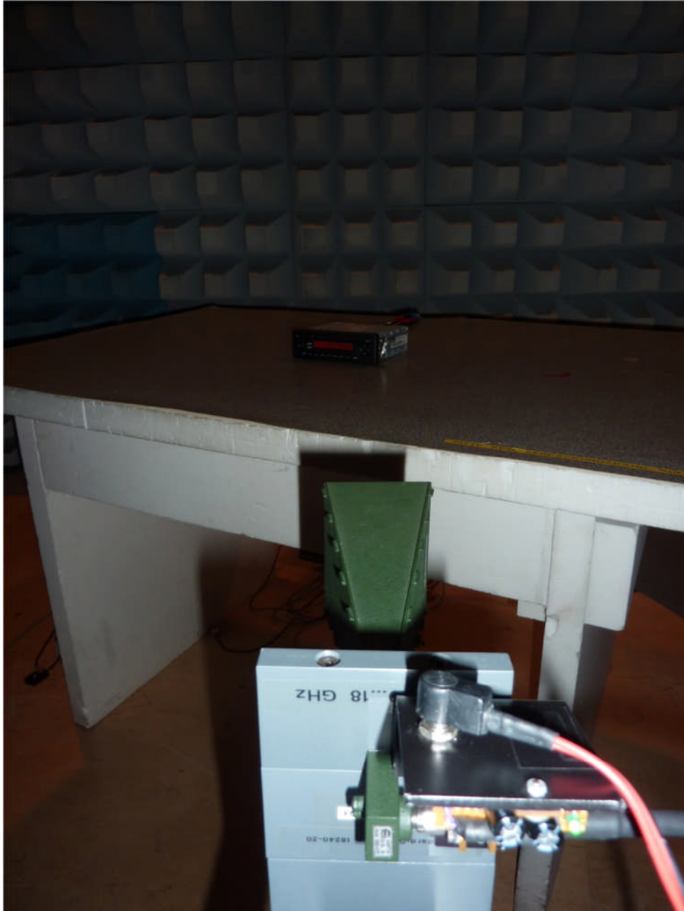
113093_10.JPG: Test setup fully anechoic chamber
