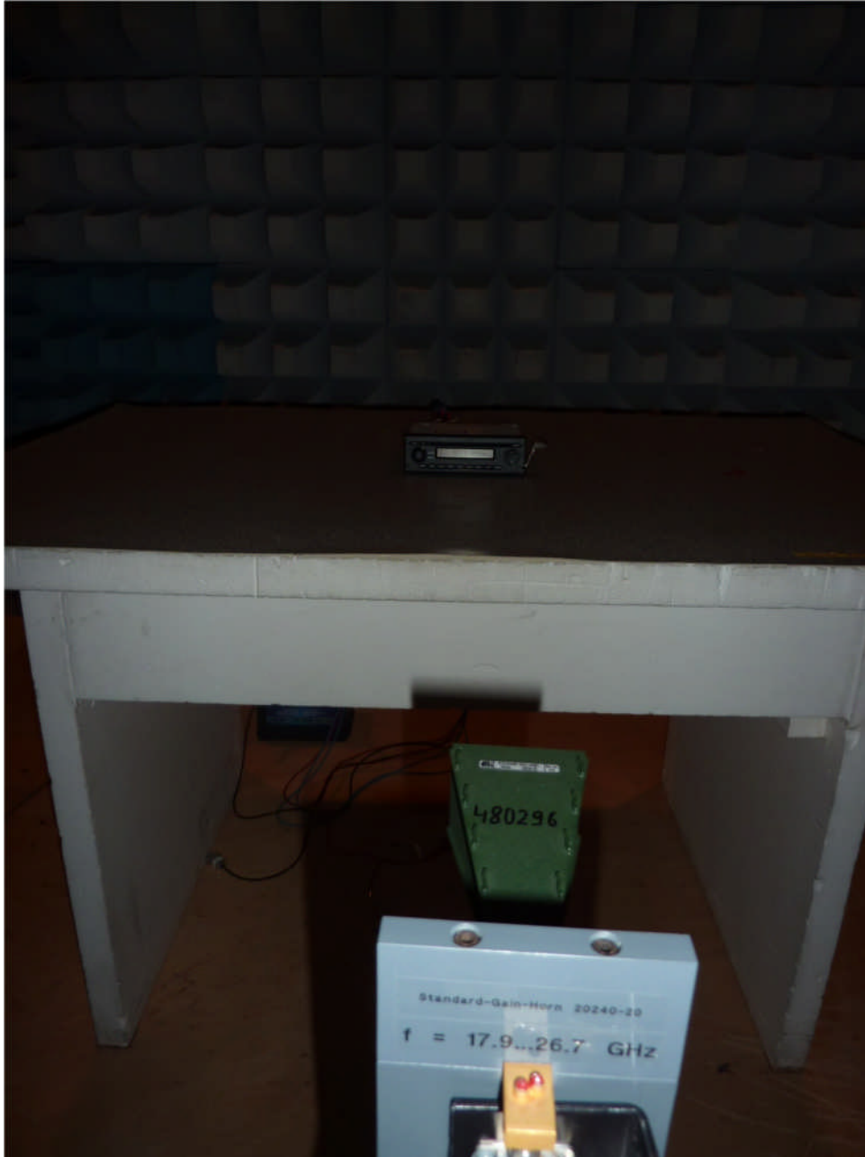
113093_11.JPG: Test setup fully anechoic chamber
