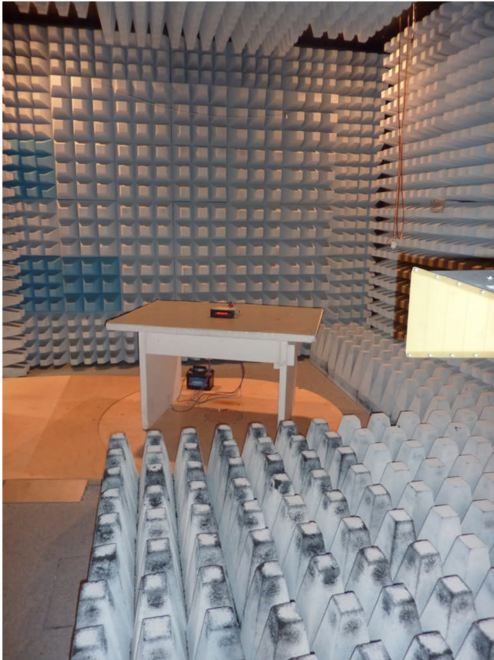
113093_09.JPG: Test setup fully anechoic chamber
