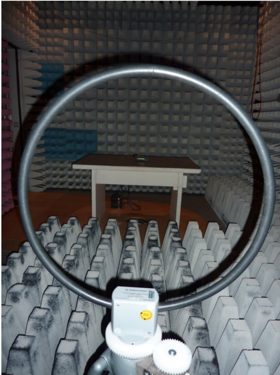
113093_13.JPG: Test setup fully anechoic chamber
