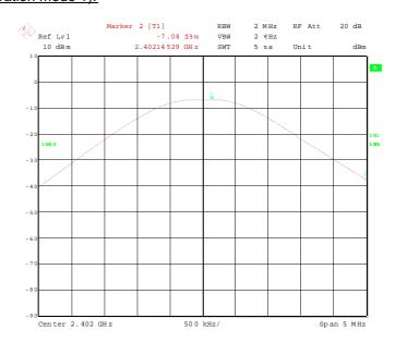
113093 59.wmf: Maximum peak output power at the middle of the assigned frequency band (operation mode 2):
