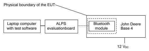
The following test modes were adjusted during the tests:
