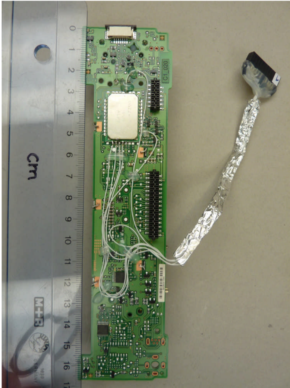
113093_EUT23.JPG: Switch PCB, rear view
