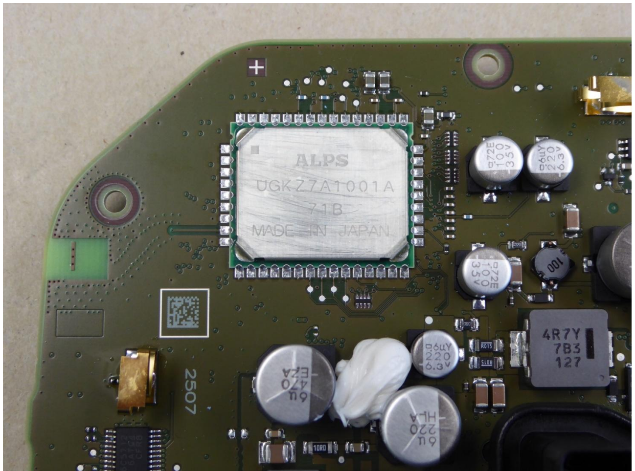
162097_18.jpg: EUT #005 – UGKZ7A1001A module – close-up
