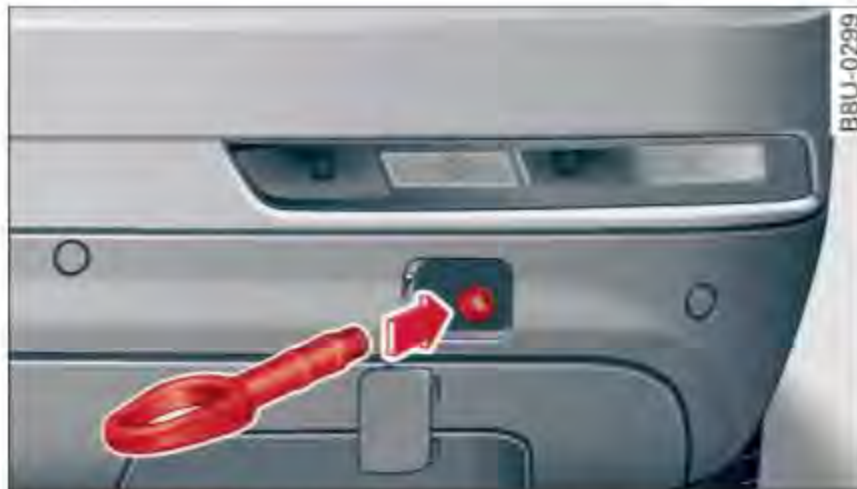
Fig. 165 Rear bumper: installing the towing loop
