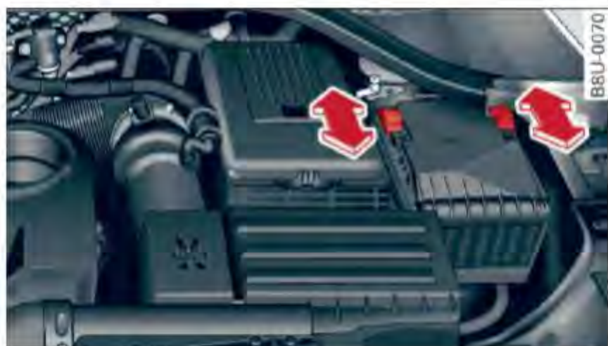
Fig. 159 Engine compartment: removing the fuse panel cover
