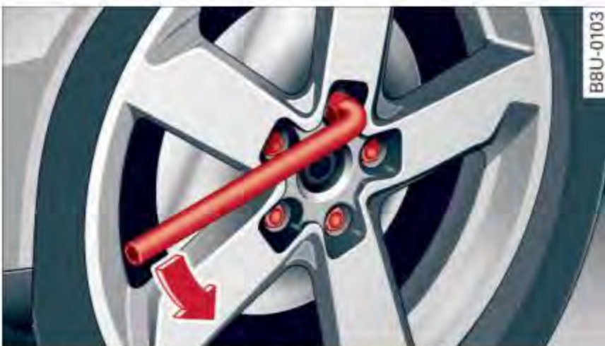
Fig. 151 Changing a wheel: loosening the wheel bolts
