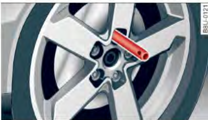
Fig. 155 Changing a wheel: alignment pin inside the top hole
