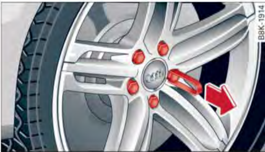
Fig. 150 Changing a wheel: removing the wheel bolt caps
