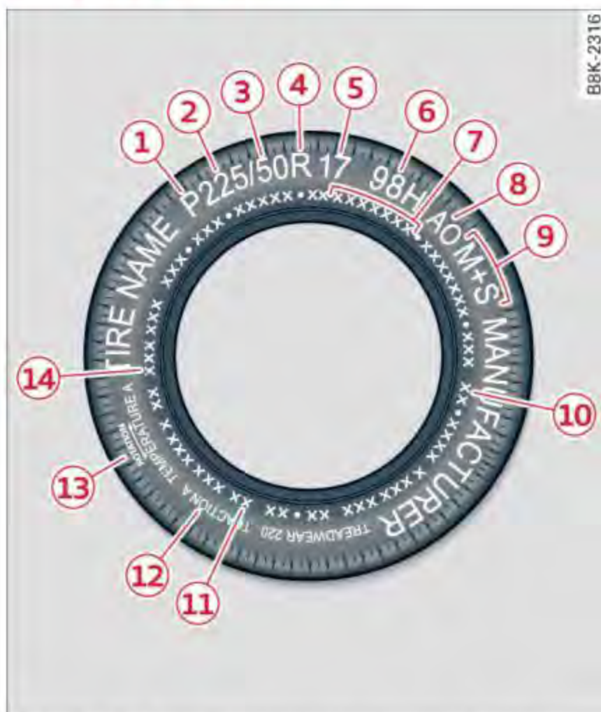
Fig. 144 Tire designations on the sidewall
