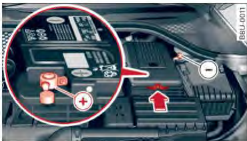
Fig. 142 Engine compartment: connectors for a charger and jump start cables
