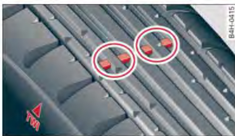
Fig. 145 Tire profile: treadwear indicator
