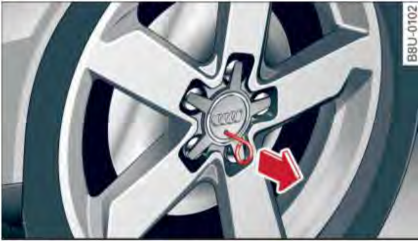
Fig. 149 Changing a wheel: removing the wheel cover
