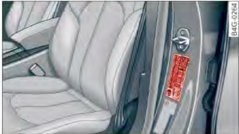
Fig. 146 Driver's side B-pillar: tire pressure label
