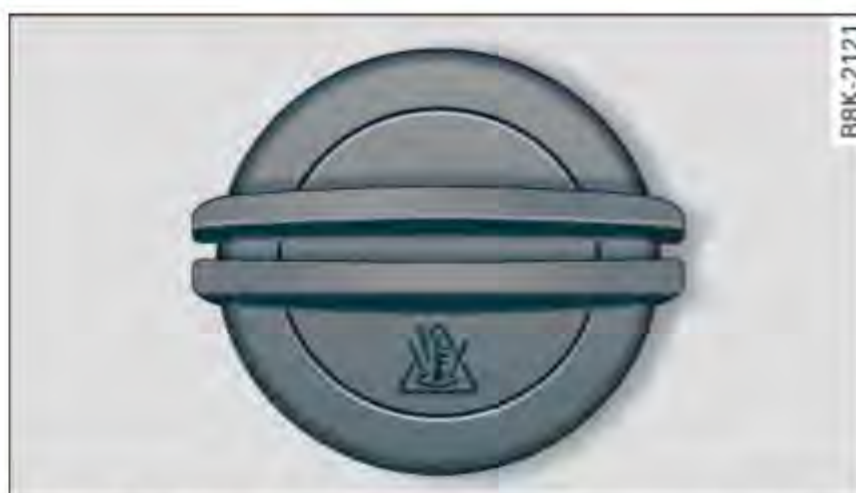
Fig. 140 Engine compartment: coolant expansion tank cover
