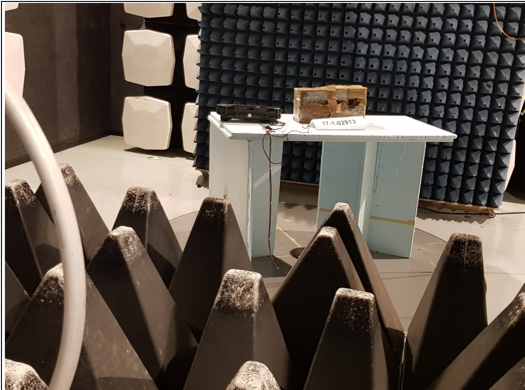
Photograph 1: Magnetic fields measurement test set-up (overview)
