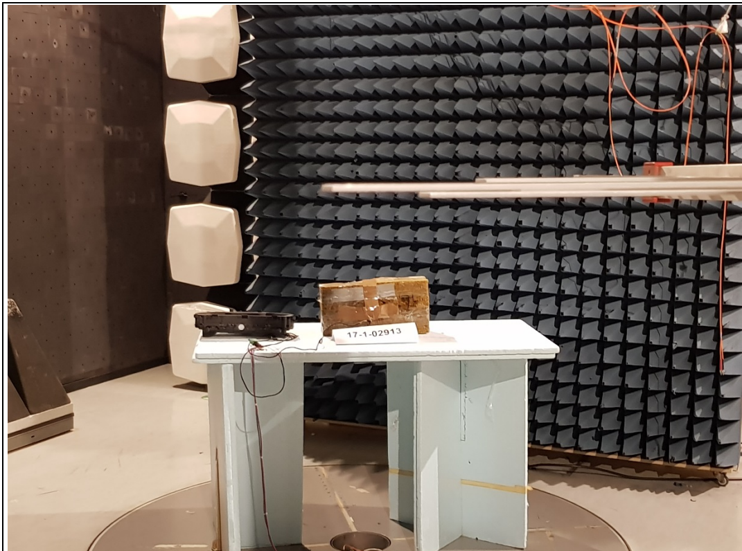
Photograph 3: Electrical field measurement test set-up (overview)
