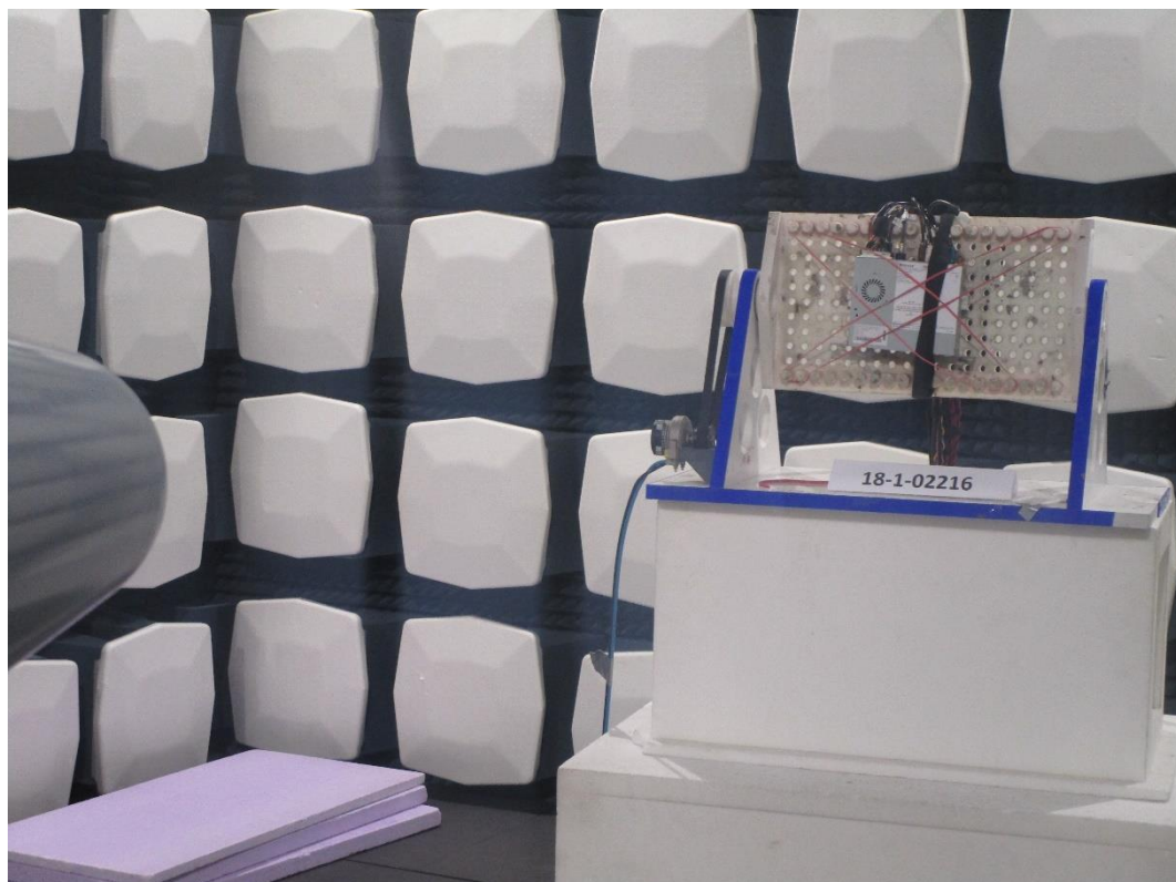
Photograph 4: Setup for Radiated emissions above 1GHz measurements, overview
