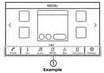
Various system functions can be accessed by touching the items on the Launch Bar ① which is displayed on most of the main menu screens. (The Launch Bar does not appear on some screens such as scrolled map screen, keyboard screen, etc.)
