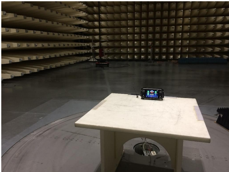
Photo 8: RSE set-up (30MHz to 1GHz)
