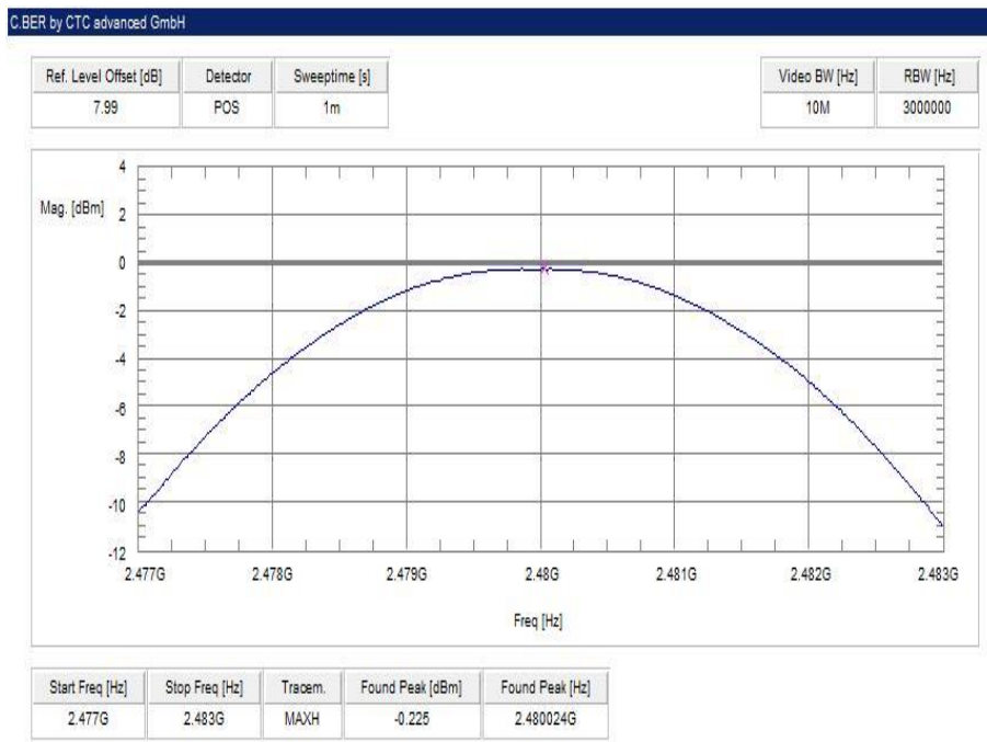
Plot 6: highest channel – 2480 MHz, Pi / DQPSK modulation
