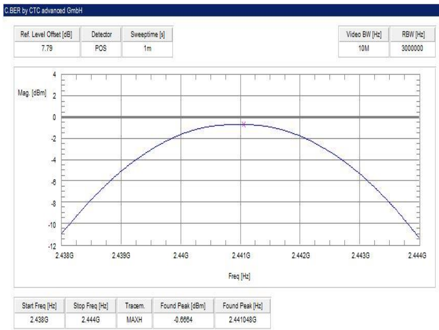
Plot 5: middle channel – 2441 MHz, Pi / DQPSK modulation
