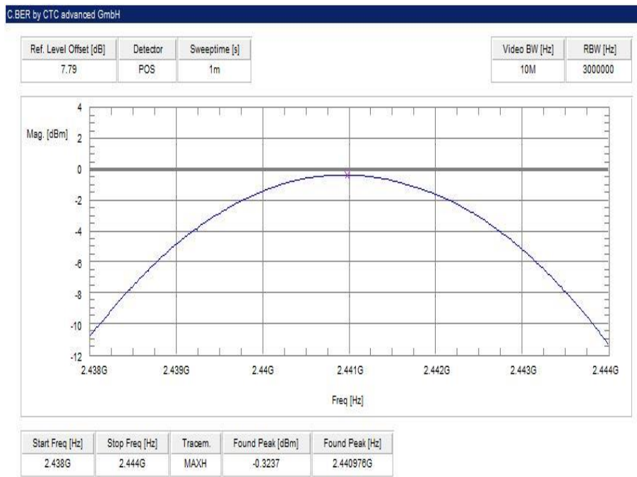
Plot 8: middle channel – 2441 MHz, 8 DPSK modulation
