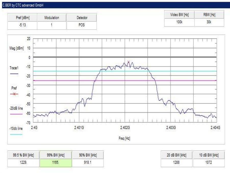
Plot 4: lowest channel – 2402 MHz, Pi / DQPSK modulation
