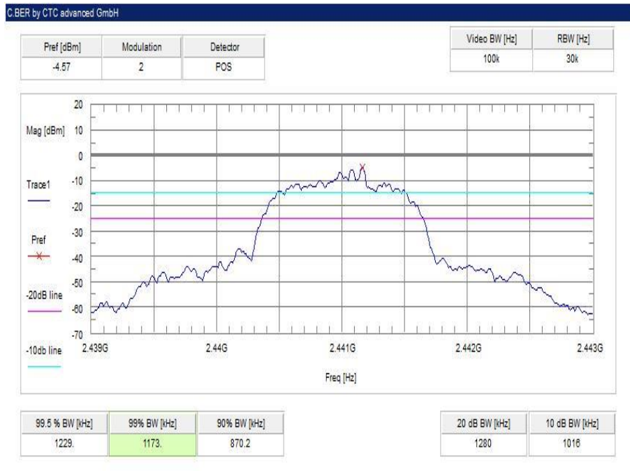
Plot 8: middle channel – 2441 MHz, 8 DPSK modulation
