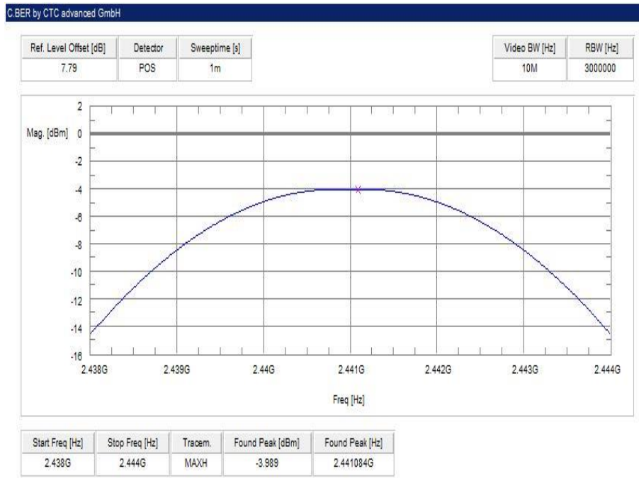
Plot 2: middle channel – 2441 MHz, GFSK modulation
