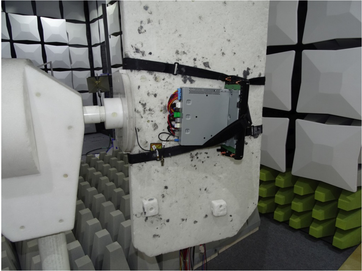
Photo 2: Test setup for radiated measurements (Enclosure, fully-anechoic chamber, 1-24 GHz intentional radiator §15)
