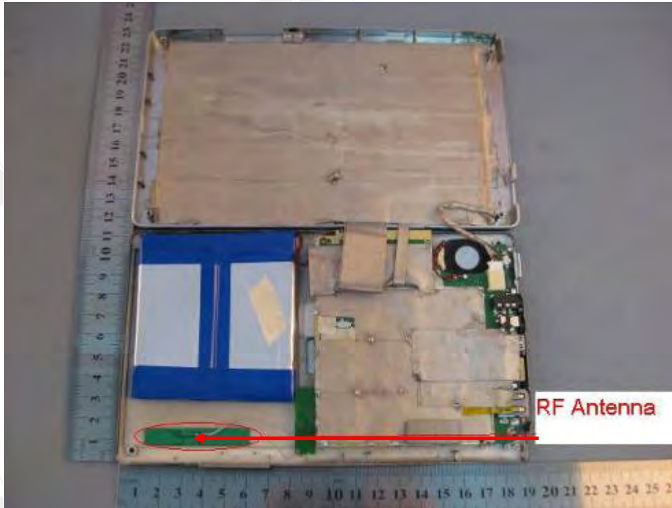
Fig.3 Antenna position of EUT
