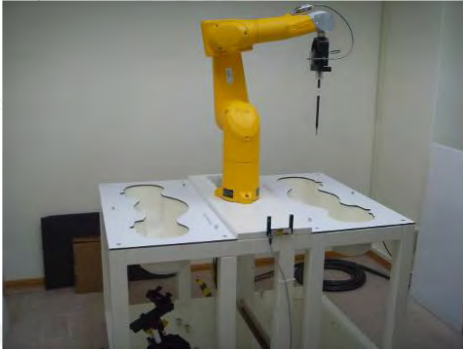
Fig.1 Photograph of the SAR measurement System
