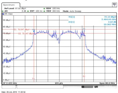
99% Occupied Bandwidth Plot on Configuration IEEE 802.11n MCS0 HT40 / 2422 MHz / Chain 1 + Chain 2
