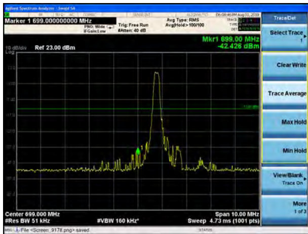
LTE Band 12 QPSK 10MHz CH-Low, 100%RB
