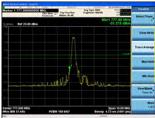
LTE Band 13 QPSK 5MHz CH-Low, 100%RB
