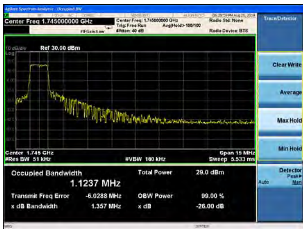
LTE Band 66 QPSK 15MHz CH-Middle
