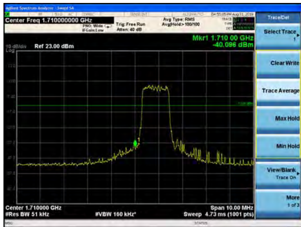
LTE Band 4 QPSK 5MHz CH-Low, 1 RB
