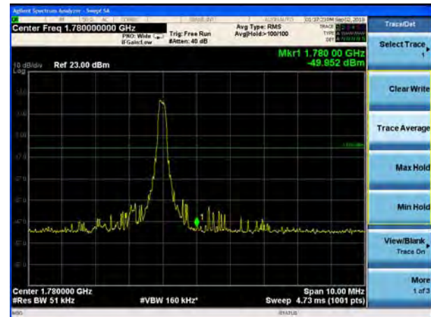
LTE Band 66 QPSK 15MHz CH-High, 1 RB
