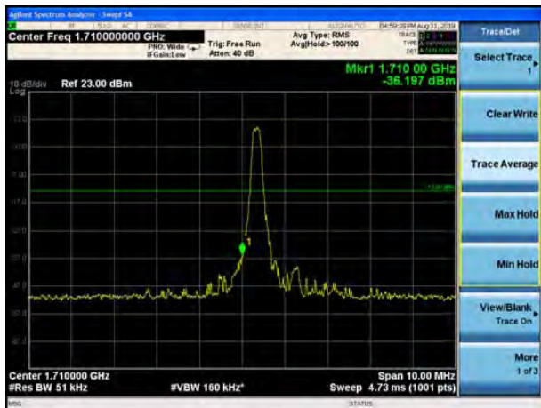
LTE Band 4 16QAM 5MHz CH-Low, 100%RB
