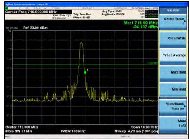
LTE Band 12 QPSK 1.4MHz CH-High, 100%RB
