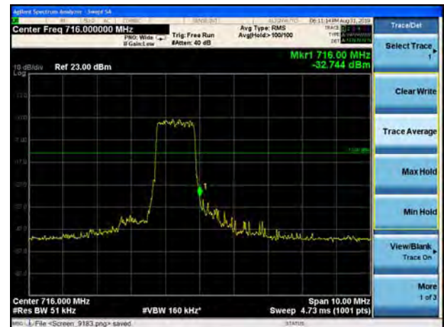
LTE Band 12 QPSK 3MHz CH-High, 1 RB
