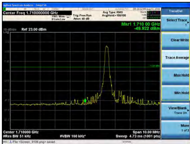
LTE Band 4 QPSK 20MHz CH-Low, 100%RB
