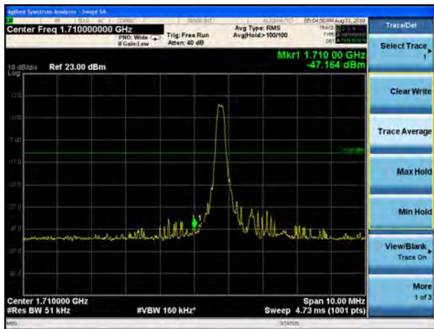
LTE Band 4 QPSK 10MHz CH-Low, 100%RB
