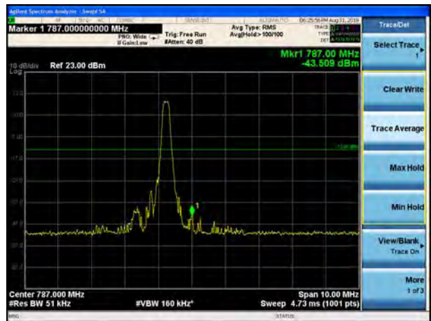
LTE Band 13 16QAM 10MHz CH- High, 100%RB
