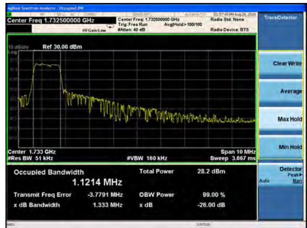
LTE Band 4 QPSK 20MHz CH-Middle
