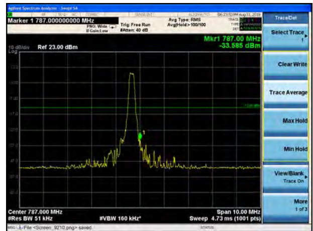
LTE Band 13 QPSK 5MHz CH- High, 100%RB
