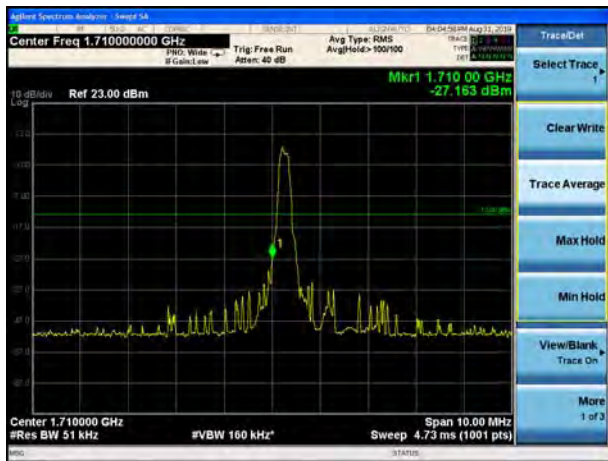
LTE Band 4 16QAM 1.4MHz CH-Low, 100%RB
