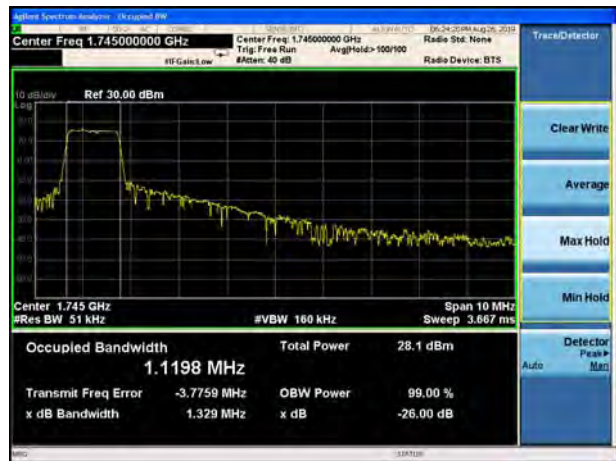
LTE Band 66 QPSK 20MHz CH-Middle
