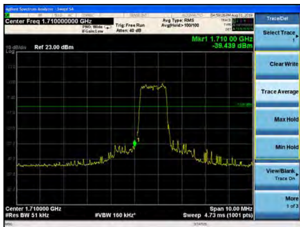
LTE Band 4 QPSK 5MHz CH-Low, 100%RB
