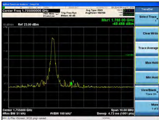
LTE Band 4 16QAM 20MHz CH-Low, 100%RB
