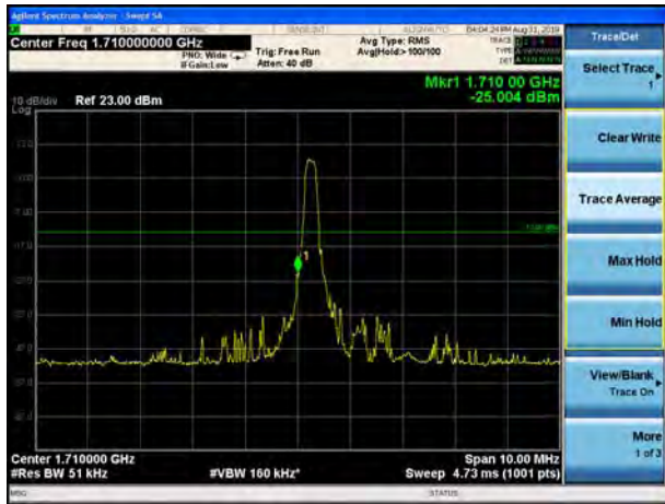
LTE Band 4 QPSK 1.4MHz CH-Low, 100%RB
