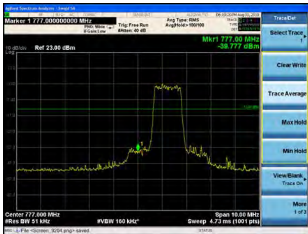
LTE Band 13 16QAM 5MHz CH-Low, 1 RB
