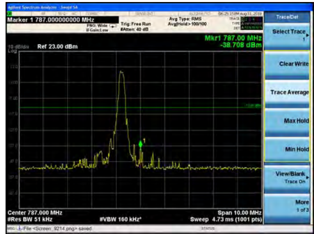
LTE Band 13 QPSK 10MHz CH- High, 100%RB
