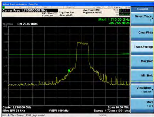
LTE Band 4 16QAM 15MHz CH-Low, 1 RB
