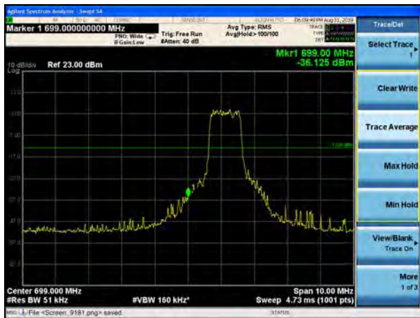
LTE Band 13 QPSK 5MHz CH-Low, 1 RB
