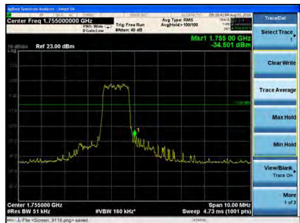
LTE Band 4 QPSK 5MHz CH-High, 100%RB
