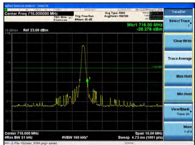
LTE Band 12 16QAM 1.4MHz CH-High, 1 RB
