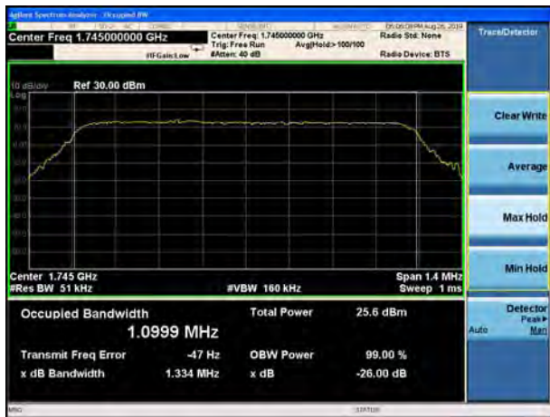
LTE Band 66 QPSK 5MHz CH-Middle
