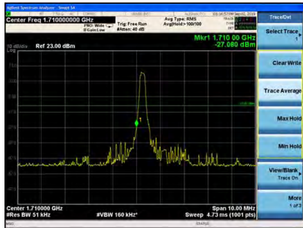
LTE Band 66 QPSK 1.4MHz CH-Low, 100%RB
