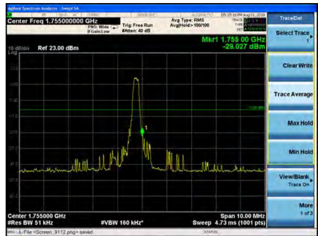
LTE Band 4 16QAM 1.4MHz CH-High, 100%RB
