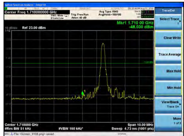
LTE Band 4 16QAM 20MHz CH-High, 100%RB
