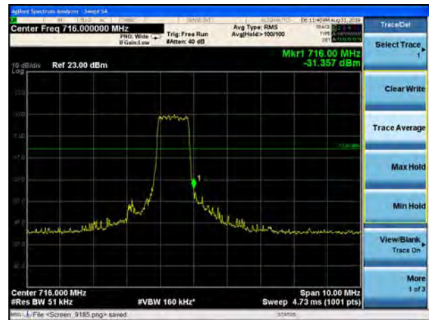
LTE Band 12 16QAM 3MHz CH-High, 1 RB
