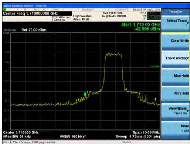
LTE Band 4 QPSK 20MHz CH-Low, 100%RB
