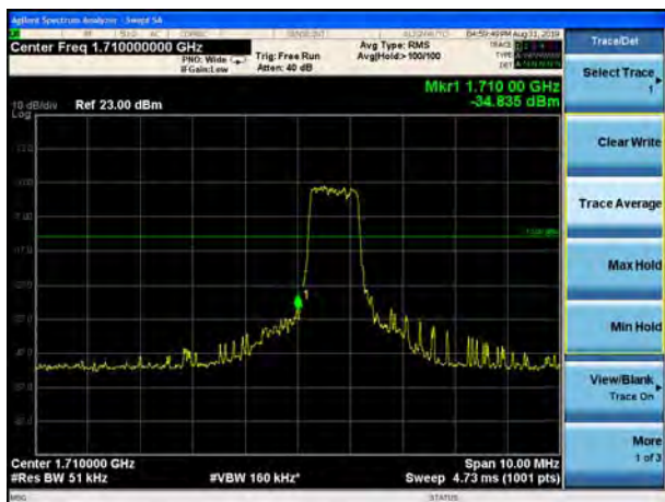
LTE Band 4 16QAM 5MHz CH-Low, 100%RB
