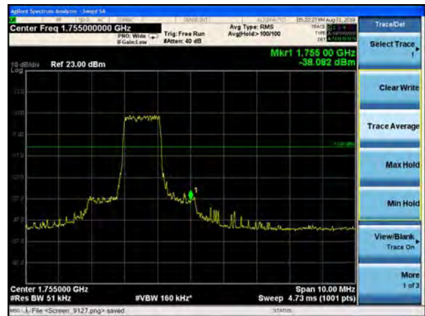
LTE Band 4 QPSK 20MHz CH-High, 1 RB
