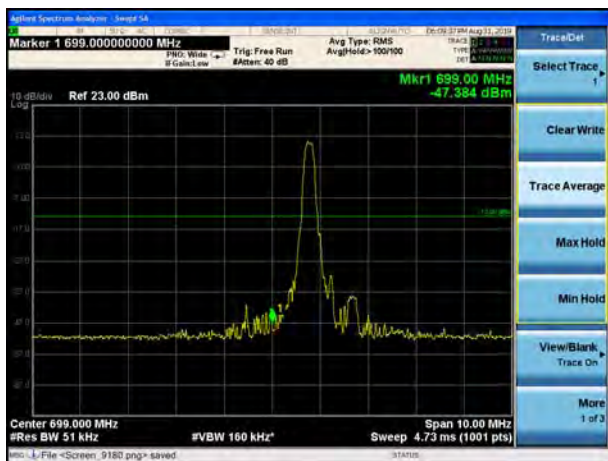
LTE Band 12 16QAM 10MHz CH-Low, 1 RB
