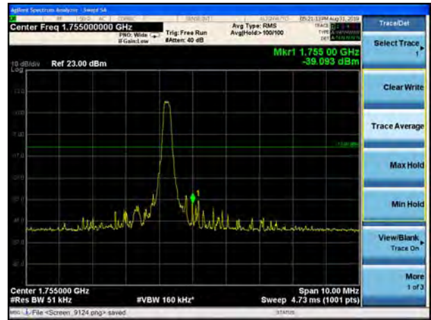
LTE Band 4 16QAM 10MHz CH-High, 100%RB
