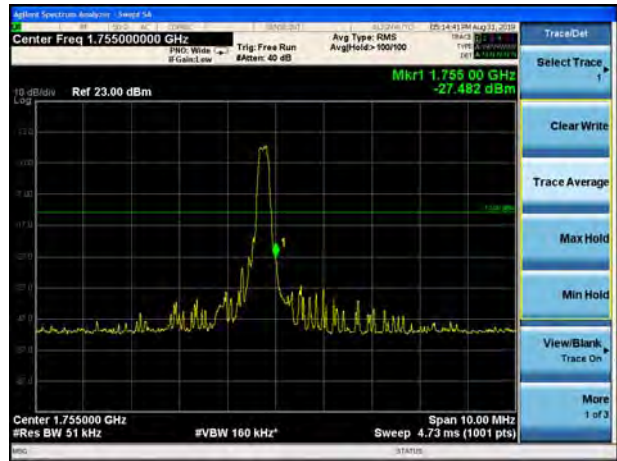
LTE Band 4 QPSK 1.4MHz CH-High, 100%RB
