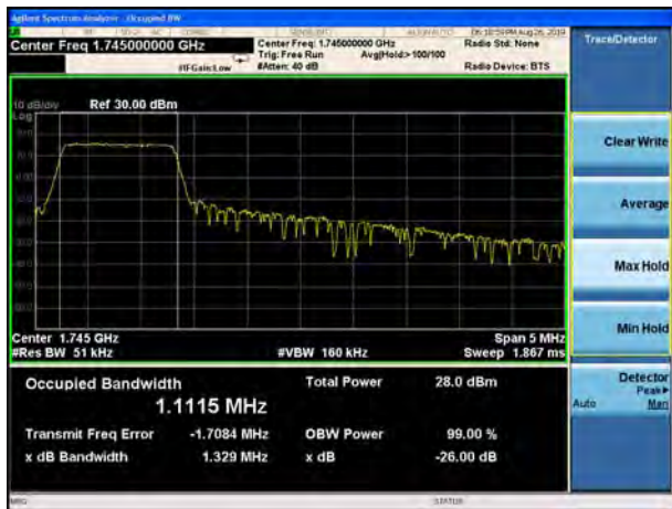
LTE Band 66 QPSK 15MHz CH-Middle
