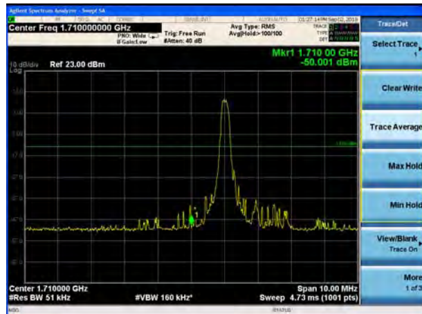
LTE Band 66 QPSK 15MHz CH-Low, 1 RB
