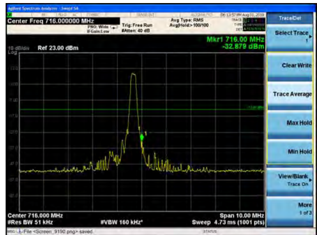
LTE Band 12 QPSK 5MHz CH-High, 100%RB
