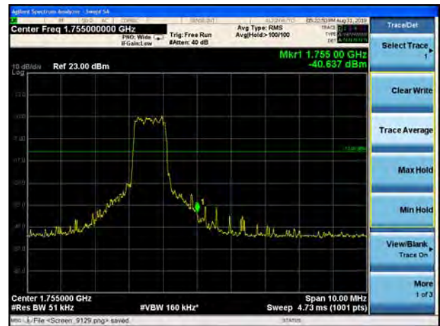
LTE Band 4 16QAM 20MHz CH-High, 1 RB
