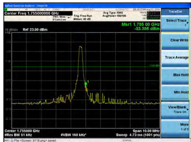
LTE Band 4 QPSK 5MHz CH-High, 100%RB
