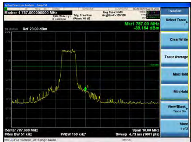
LTE Band 13 16QAM 5MHz CH-High, 1 RB
