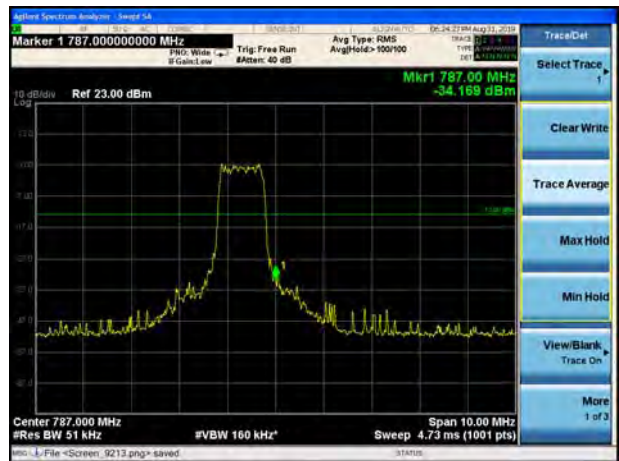
LTE Band 13 16QAM 10MHz CH-High, 1 RB
