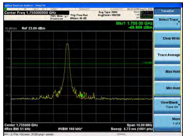
LTE Band 4 16QAM 15MHz CH-High, 1 RB
