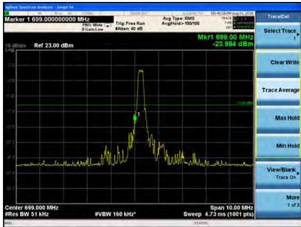
LTE Band 12 QPSK 1.4MHz CH-Low, 100%RB
