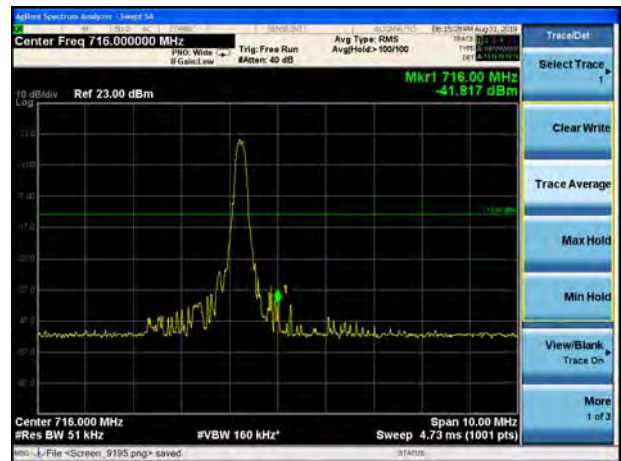
LTE Band 12 QPSK 10MHz CH-High, 100%RB
