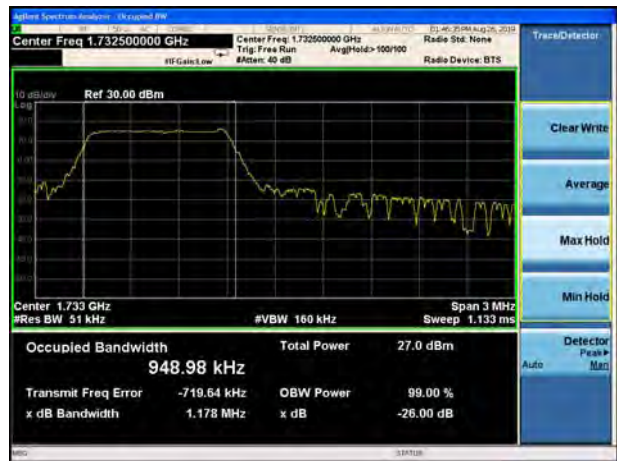
LTE Band 4 16QAM 10MHz CH-Middle
