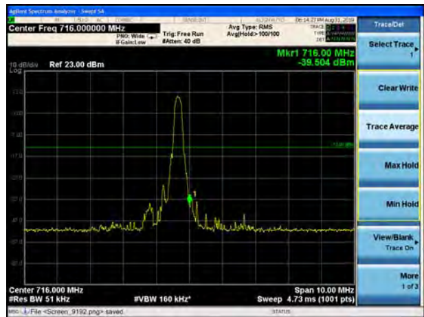
LTE Band 12 16QAM 5MHz CH-High, 100%RB
