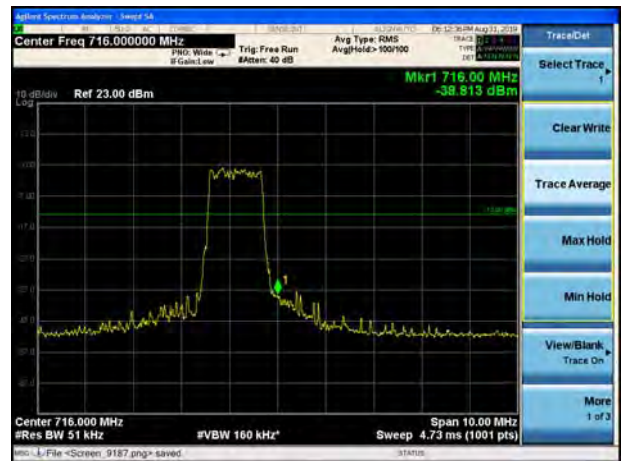
LTE Band 12 QPSK 5MHz CH-High, 1 RB
