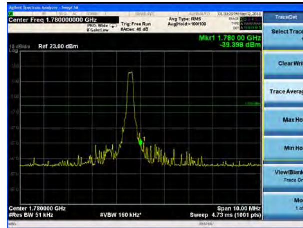
LTE Band 66 QPSK 3MHz CH-High, 1 RB
