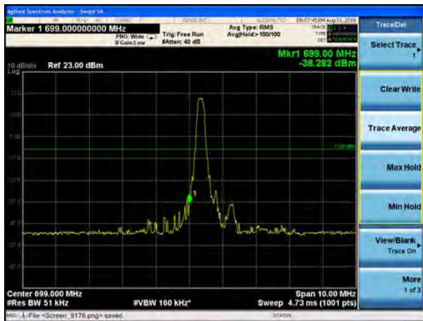
LTE Band 12 16QAM 5MHz CH-Low, 100%RB
