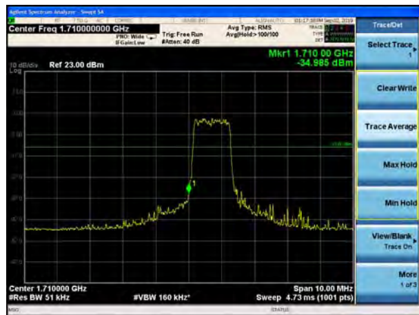
LTE Band 66 QPSK 3MHz CH-Low, 1 RB
