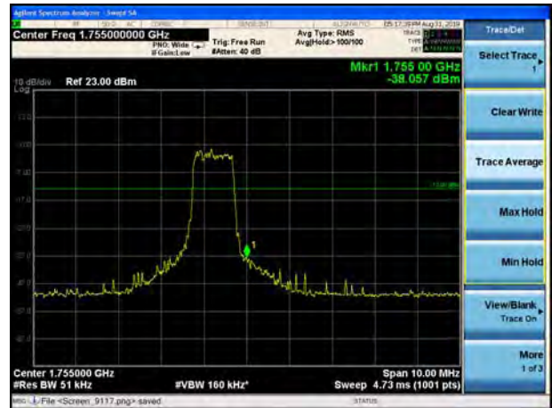
LTE Band 4 16QAM 5MHz CH-High, 1 RB
