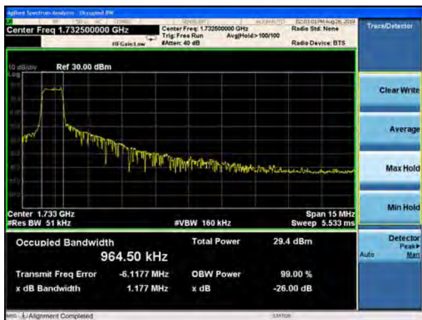
LTE Band 4 16QAM 15MHz CH-Middle
