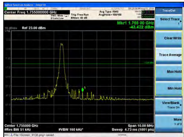
LTE Band 4 QPSK 20MHz CH-High, 100%RB
