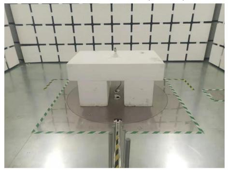
**1.2** Unwanted Emissions that fall Outside of the Restricted Bands(Radiated) and Unwanted Emissions in the Restricted Bands (Radiated) above 1GHz
