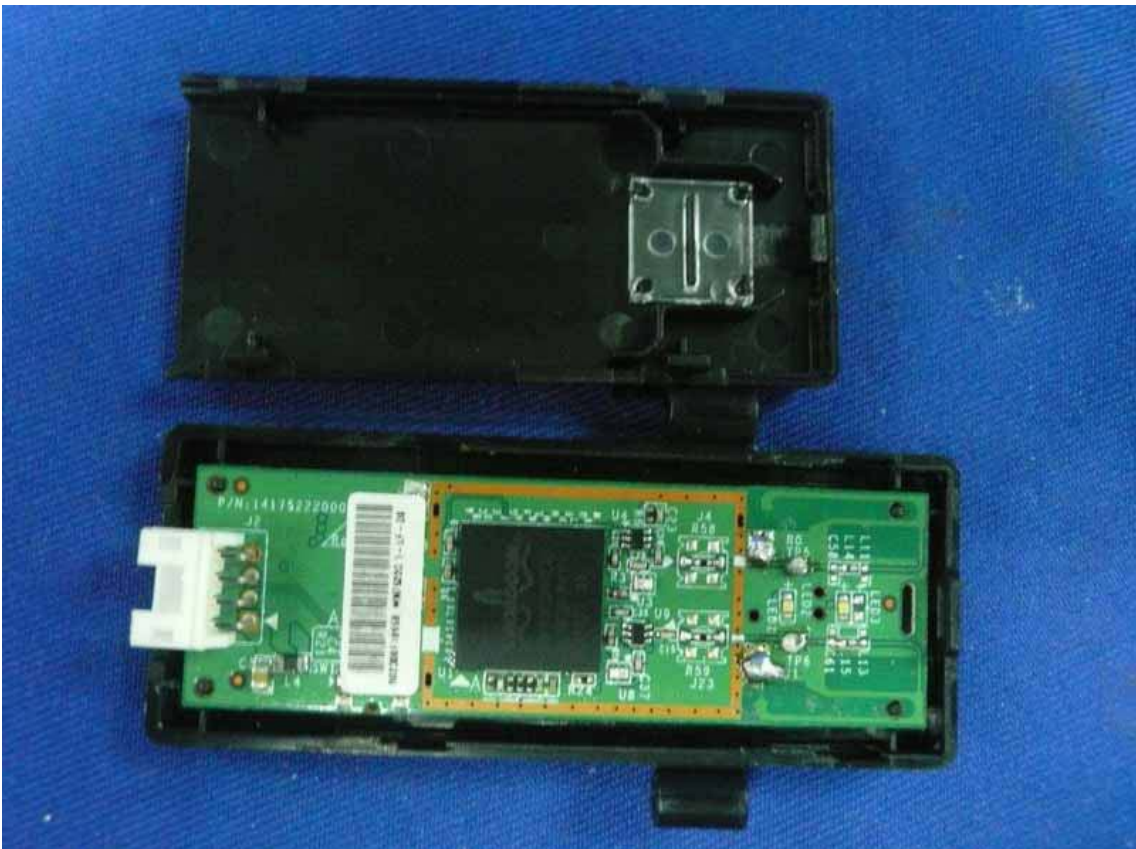
Figure 12 Inside of the EUT
