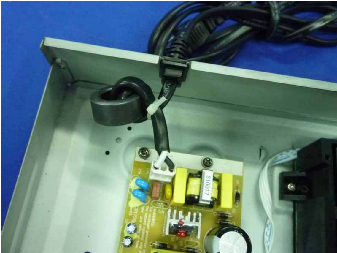
Figure 5 Inside of the EUT
