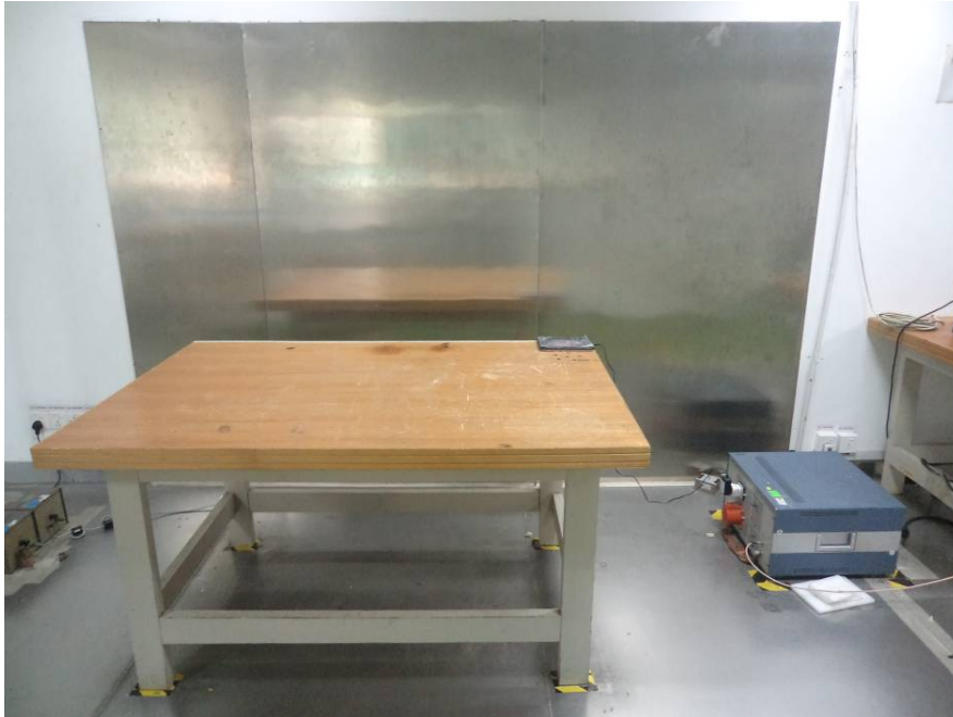
Conducted Emissions - Front View
