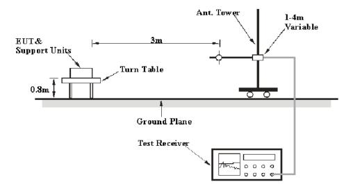
The radiated emission tests were performed in the 3 meters test site, using the setup accordance with the ANSI C63.4-2009. The specification used was the FCC Part 15.109 Class B limits.
