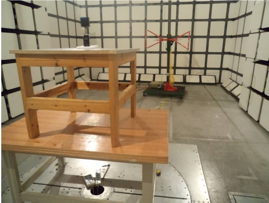
Transmitting Radiated Emissions (Below 1 GHz)
