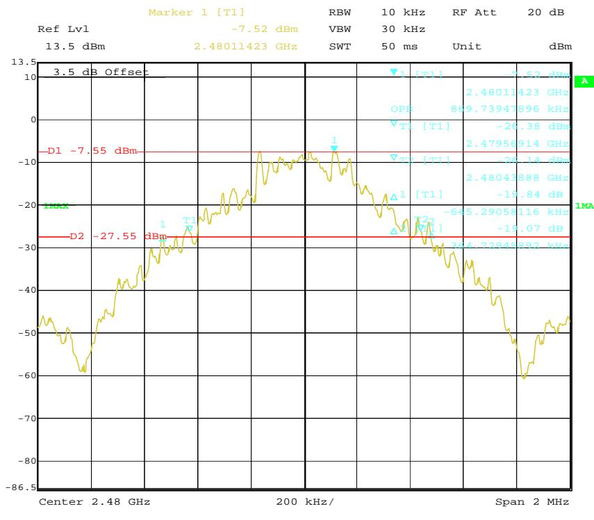
**EDR ( $\pi/4$ -DQPSK): Low Channel**
