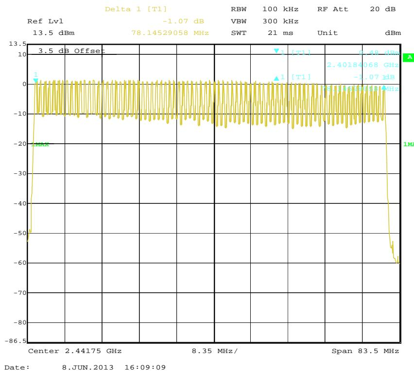
**EDR ( $\pi/4$ -DQPSK): Number of Hopping Channels**
