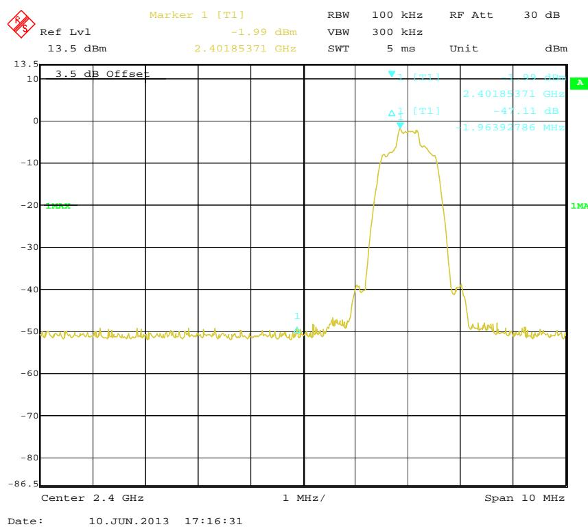
**EDR ( $\pi/4$ -DQPSK): Band Edge-Right Side**
