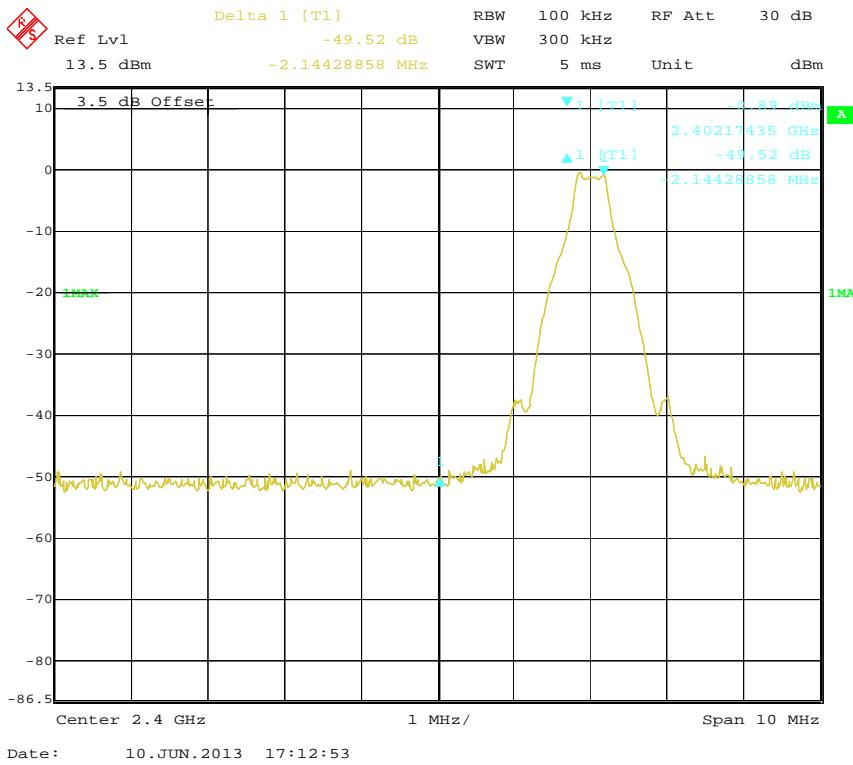
**BDR (GFSK): Band Edge-Right Side**
