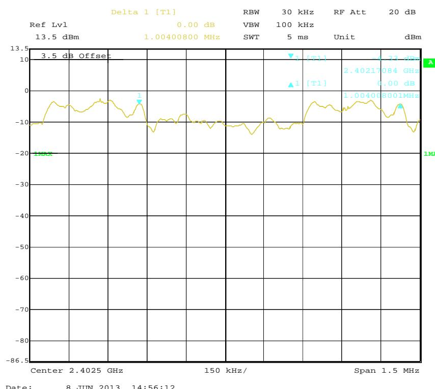
**EDR ( $\pi/4$ -DQPSK): Middle Channel**
