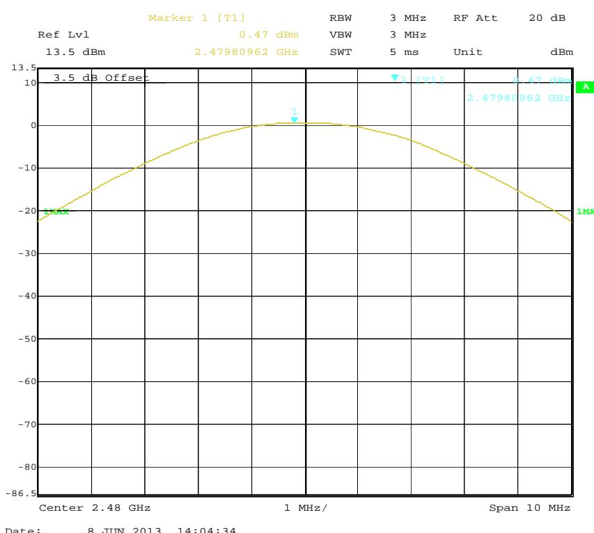
**EDR( $\pi/4$ -DQPSK): Low Channel**
