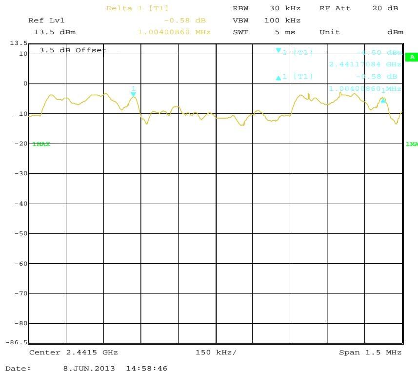
**EDR ( $\pi/4$ -DQPSK): High Channel**
