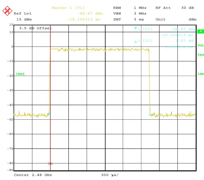
**Pulse time, Low Channel, DH5**
